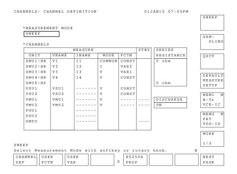
On the "CHANNELS: CHANNEL DEFINITION" screen, you define the measurement mode and how to use each channel.
