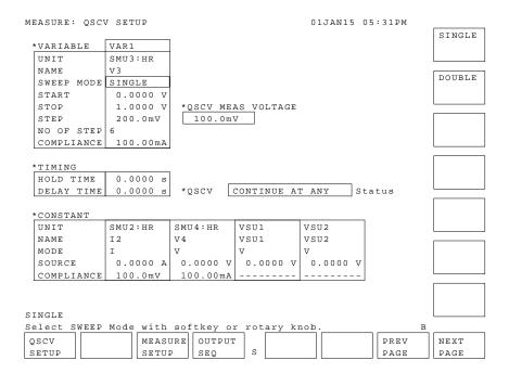
On this screen, you set the output parameters for each unit used in the quasi-static CV measurements.
