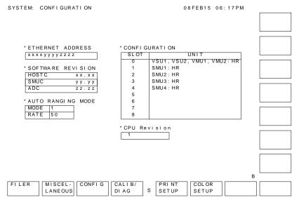
The SYSTEM: CONFIGURATION screen contains the system firmware revision and hardware configuration for the 4155C/4156C.
