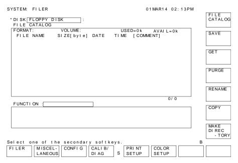
On the "SYSTEM: FILER" screen, you can execute file operations from a diskette, internal memory, or the network file system.
