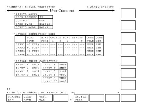
The 4155C/4156C can control the Agilent E5250A Low Leakage Switch Mainframe if it has an E5252A matrix card installed. On the "CHANNELS: E5250A PROPERTIES" screen, you can define the E5250A setup and the connection modes for the E5252A.
