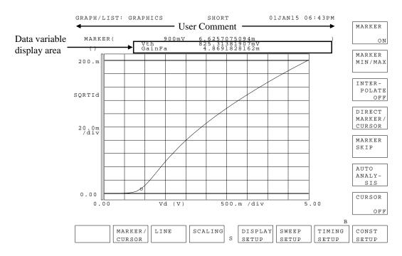
On the "GRAPH/LIST: GRAPHICS" screen, measurement results are displayed, and you can analyze the measurement results graphically.
