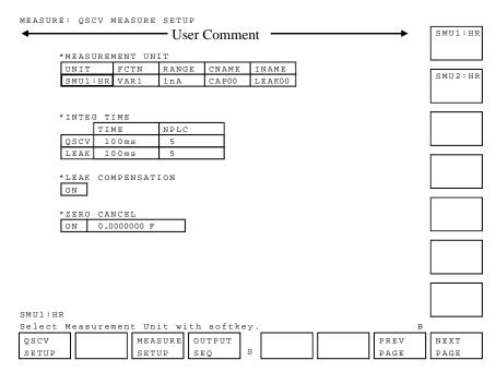
On the "MEASURE: QSCV MEASURE SETUP" screen, you select the measurement units, range, integration time, leakage current compensation, and QSCV zero cancel.
