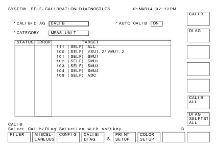
The SYSTEM: SELF-CALIBRATION/DIAGNOSTICS screen is used to execute self-calibration and diagnostics.
