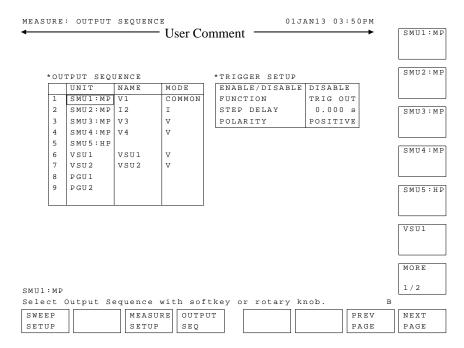
On this screen, you set the output sequence and triggering parameters for measurement state.
