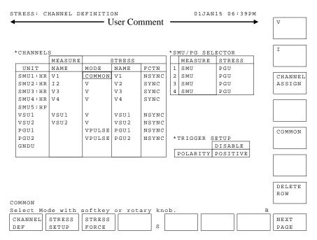
On the "STRESS: CHANNEL DEFINITION" screen, you define how to use the channels for stress force, how to control the SMU/PG selector, and trigger usage in the stress force state.
