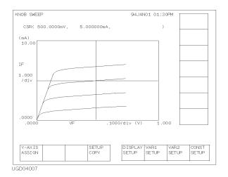
To start the knob sweep measurement, press the green key and then the Single front-panel key. The 4155C/4156C displays KNOB SWEEP screen, and starts measurements. To stop the knob sweep measurement, press the Stop front-panel key or a PAGE CONTROL group key.
