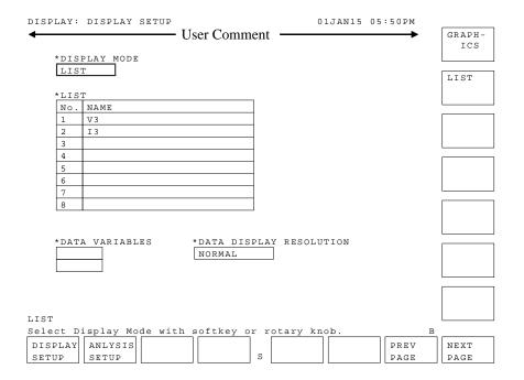
On the "DISPLAY: DISPLAY SETUP" screen for list results, you enter variable names for which you want results to be displayed numerically. The measurement channels are determined by the variable names that you set on this screen.
