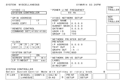
The SYSTEM: MISCELLANEOUS screen contains miscellaneous settings for the 4155C/4156C.
