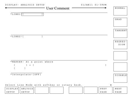
On the "DISPLAY: ANALYSIS SETUP" screen, you set up the automatic analysis function. When a measurement finishes, the function automatically draws lines, a marker, or both as specified on this screen.
