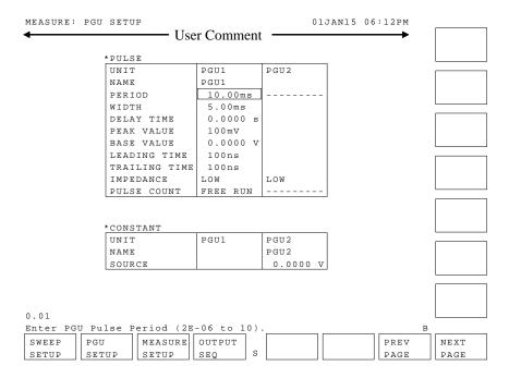
On the "MEASURE: PGU SETUP" screen, you set output parameters for each PGU. For more information about PGUs, see *User's Guide: Measurement and Analysis*.
