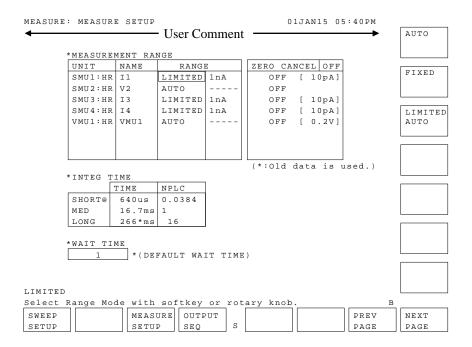
On the "MEASURE: MEASURE SETUP" screen, you set measurement range, zero cancel, integration time, and wait time.
