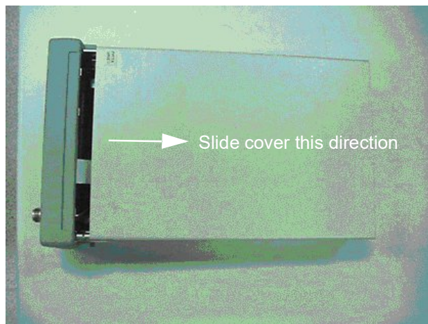
Figure A-3 Remove the power meter cover
