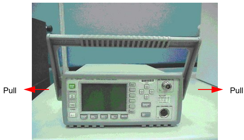
Figure A-2 Remove the power meter handle
