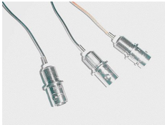
Figure A-7 Solder each wire onto the screw-fit BNC female connectors
