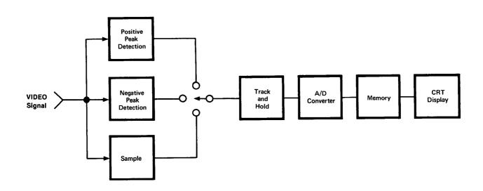
During a sweep, only a specified amount of time is available for writing data into each of the 1001 trace memory addresses. In two of these time periods, the positive and negative peak detectors obtain the maximum and minimum IF signal excursions, respectively, and store these values in *alternate* trace memory addresses. This technique allows a graphic presentation of noise on the CRT display.
