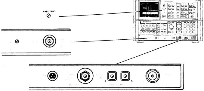
Either of the RF signal inputs can be selected: INPUT 1: 100 Hz to 1500 MHz, dc coupled, BNC fused  $50\Omega$ . INPUT 2: 100 kHz to 1500 MHz, ac coupled, Type N  $50\Omega$ . Isolation between inputs is >90 dB.
