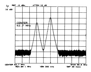
The number of significant digits in the readout depends on the frequency span selected. The narrower the span, the more significant digits.
