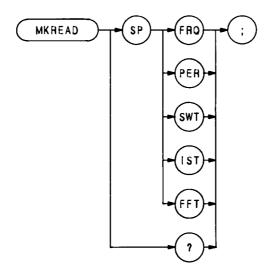
The MKREAD command selects the type of active trace information displayed by the analyzer marker readout: marker frequency, period, sweep time, inverse sweep time, or fast fourier transform readout.
