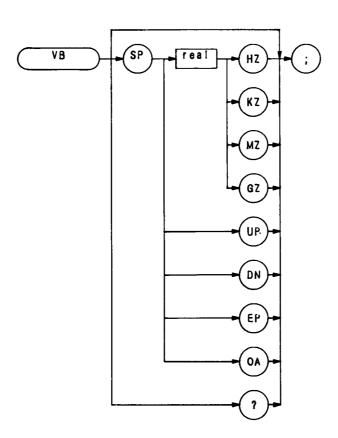
The VB command specifies the video filter bandwidth, which is a post-detection filter. Available bandwidths are 1 Hz, 3 Hz, 10 Hz, 30 Hz, 100 Hz, 300 Hz, 1 kHz, 3 kHz, 10 kHz, 30 kHz, 100 kHz, 1 MHz, and 3 MHz.
