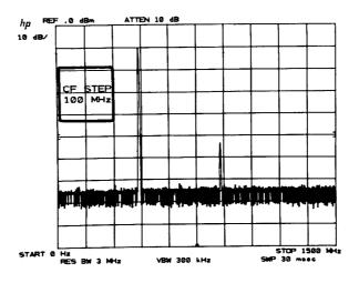
When the center frequency is activated with step size in MANUAL, the active function readout includes both the center frequency and the step size value.
