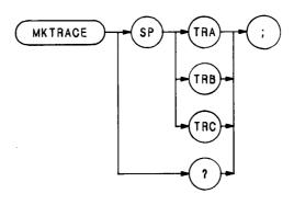
The MKTRACE command moves the active marker to a corresponding position in trace A, B, or C.
