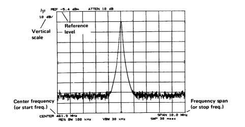
The COUPLED FUNCTIONS that describe the swept receiver characteristics of the spectrum analyzer are:
