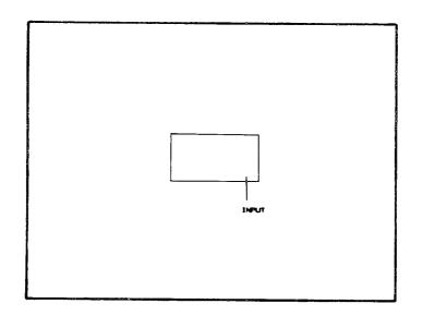
The label "INPUT" can be made to blink by adding blink on (bk on) and blink off (bk of) words before and after the "INPUT" label.
