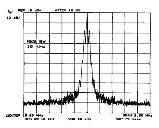
Reduce the resolution bandwidth without changing the span with 🐨 🔿 . (The DATA knob 🔘 or number/units keyboard could also have been used.)
