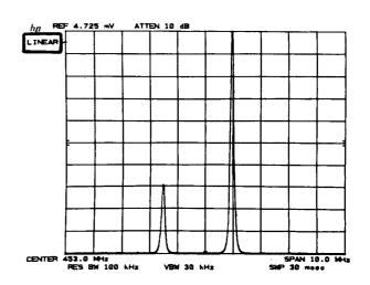
In LINEAR, a specific voltage per division scale can be set by entering a voltage reference level value. For example, to set the scale to 3 mV/division, key in 30 mV reference level. (Voltage entries are rounded to the nearest 0.1 dB, so the 30 mV entry becomes 30.16 mV, which equals -17.4 dBm.)
