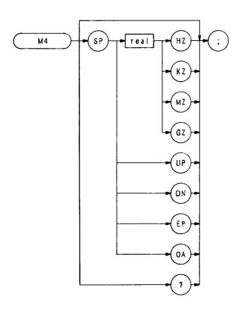
The M4 command activates a single marker at center frequency, the DATA knob changes the position of the marker and the STEP keys change the frequency span and sets the center frequency equal to the marker frequency. The functions of the M4 command and the front panel Marker Mode we are identical.
