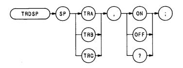
The TRDSP command displays a trace or turns if off. The command does not affect any other trace operations.
