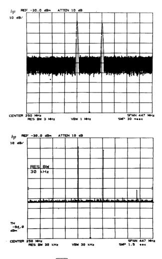
Reduction of the noise level by 10 dB (increased sensitivity) is achieved by decreasing the bandwidth by a factor of 10.
