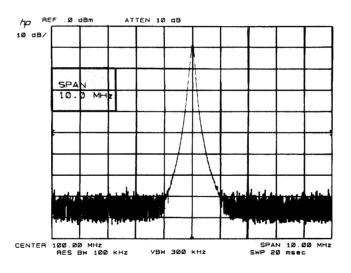
The last function activated, SPAN, will appear with its current value on the analyzer CRT as shown in the shaded box.
