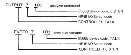
The read/write address of the HP 8568B can be changed from the front panel or via HP-IB by using the shift function P.
