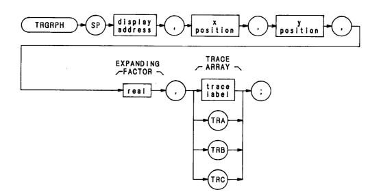
The TRGRPH command displays a trace A, B, or C, or a user-defined trace anywhere on the spectrum analyzer display. The X and Y positions orient the trace above and to the right of a point on the CRT, specified by the display address. The trace can be expanded, according to the scale determined by the expanding factor.
