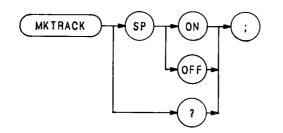
The MKTRACK command keeps the active marker at the center of the display. To keep a drifting signal at center screen, place the active marker at the desired signal before executing MKTRACK. (See MT1 and MTØ. Also see WHAT key in Section I.)
