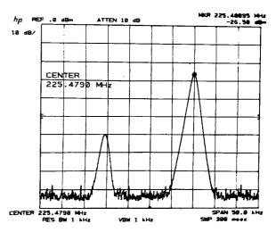
Note that the marker seeks the maximum trace response, no matter what the cause of the response. A larger signal, or the local oscillator feedthrough, would also have attracted the marker.
