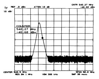
If the marker is not in the top 6 divisions, the display readout "CNTR" in the top right-hand marker area blinks, indicating the reading may be in error.
