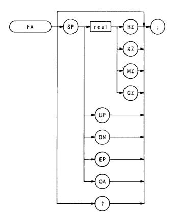
The FA command specifies the start frequency value. The function is identical with that of the front panel (start frequency value. The program line below illustrates command syntax.
