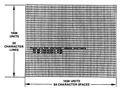
Display memory is set up to contain 64 character spaces per line with respect to display size 1. When using the third and fourth display sizes, a label can only be a maximum of 44 characters. The remaining 20 characters of the label will be stored in display memory, but will not show up on the CRT display due to the expansion of D3 and bex. At character space 65, an automatic carriage-return and line-feed will occur, at which point labeling will continue to be written on the CRT display.
