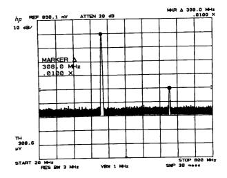
With the display referenced and scaled as shown, the readout ".0100X" designates the fractional harmonic content. Percent is calculated as 100X(.0100) = 1.0%.
