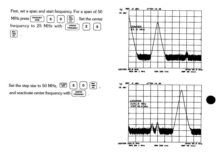
Now each sets the center frequency to the next 50 MHz span for a span-by-span surveillance of the spectrum. (Center frequency = 25 MHz, 75 MHz, 125 MHz, etc.) Center frequency step size can also be defined by the marker. See the MARKER ENTRY portion of Chapter 6.
