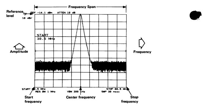
CRT GRATICULE SCALING WITH FUNCTION READOUTS
