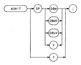
The AUNITS command sets the amplitude readouts (reference level, marker, display line, and threshold) to the specified units. (See KSA, KSB, KSC, and KSD.)
