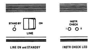
Upon LINE ON, the analyzer will perform an automatic internal instrument check, designated by the red INSTR CHECK indicators. Both LED's will turn on momentarily during the brief check routine and, if the instrument is operating properly, will go off during operation, except when another instrument check is triggered by an Instrument Preset. If one or both LED's remain on, refer to Section II, Performance Tests, in the HP 8566B/8568B Service Manual.
