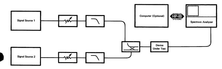
Figure 1. Test Setup for Third Order IMD Measurements
