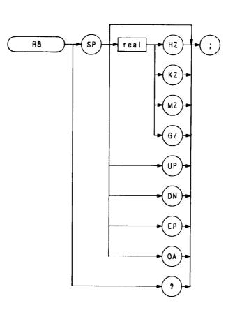
The RB command specifies the resolution bandwidth. Available bandwidths are 10 Hz, 30 Hz, 300 Hz, 1 kHz, 3 kHz, 30 kHz, 100 kHz, 300 kHz, 1 MHz, and 3 MHz. The resolution bandwidths, video bandwidths, and sweep time are normally coupled. Executing RB decouples them. Execute CR to reestablish coupling.
