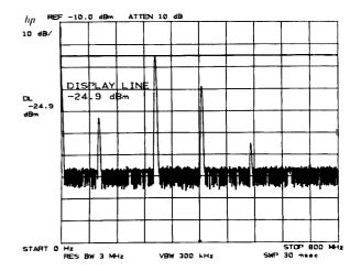
Moving the display line to each signal reads out its peak amplitude.
