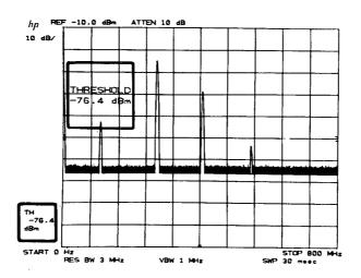
The threshold can be positioned anywhere within the graticule. It operates on TRACE  $\frac{CEEAB}{MOL}$ , or  $\overline{CEEAB}$ , TRACES A, B, and C simultaneously. When activated after LINE power ON or  $\overline{CEEBE}$ , the threshold is placed 1 division from the bottom graticule.
