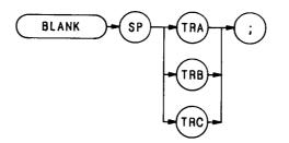
The BLANK command blanks trace A, B, or C and stops the sweep; the trace is not updated.
