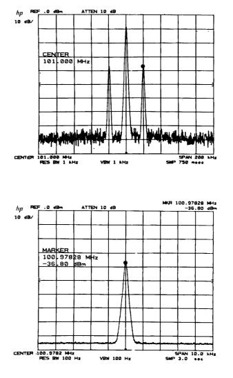
As the carrier frequency is changed, the sideband response will remain in the center of the display. Both the center frequency and marker frequency read out in the sideband's frequency.
