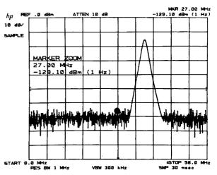
The noise level measurement readout is corrected for the analyzer's log amplifier response and detector response. The value is also normalized to a 1 Hz bandwidth.
