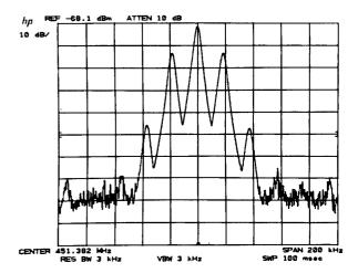
Linear scaling enables observation of the sidebands proportional to the carrier.
