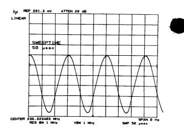
If the level does not cause a trigger within 25 msec, the sweep is triggered anyway to ensure a display. Note that this is true only for sweep times  $\leq 10$  msec.
