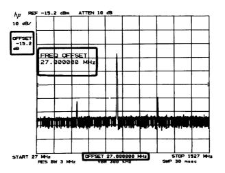
DATA entry from the keyboard can be in Hz, kHz, MHz, or GHz for frequency offset and in dB, -dB, mV, or  $\mu V$  for amplitude offset. The amplitude offset readout is always in dB. An amplitude offset entry in voltage is converted to dB offset.
