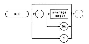
The KSG command enables video averaging. During video averaging, two traces are displayed simultaneously. Trace C contains signal responses as seen at the input detector. Trace A or B contains the same responses digitally averaged. The digital reduces the noise floor level, but does not affect the sweep time, bandwidth, or any other analog characteristics of the analyzer.
