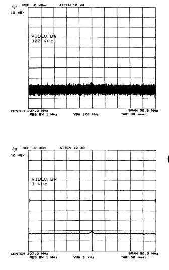
Narrowing the video bandwidth clarifies the signal and allows its amplitude measurement.
