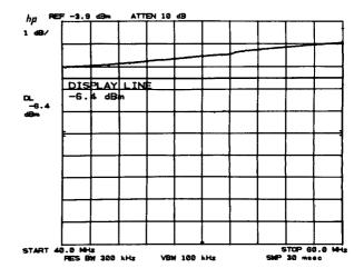
The difference between the display line (in display units) and the source/analyzer response is stored in trace B with  $\left[\begin{smallmatrix} \mathbf{u}-\mathbf{h}\\ \mathbf{u} \end{smallmatrix}\right]$ .
