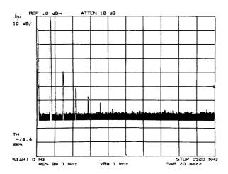
The trace data that would have been shown between display addresses 100 and 500 is omitted and the data for addresses 501 - 1001 is displayed at x positions 100 through 600.
