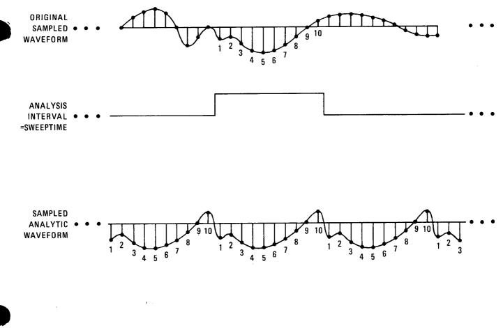
The TWNDOW command allows the source trace array to be modified so the amplitude of the trace endpoints gradually diminish to zero.
