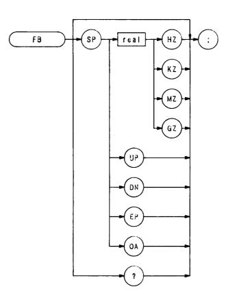
The FB command specifies the stop frequency value. The function is identical with that of the front panel key. The program below illustrates command syntax.
