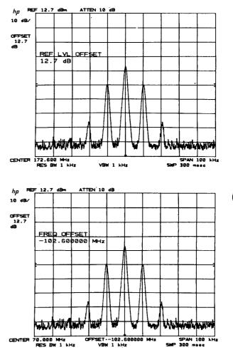
Frequency offset is entered as a negative value since the input frequency to the converter is lower than the output.
