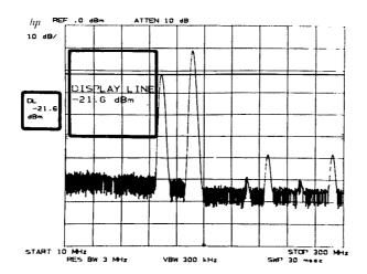
The display line can be positioned anywhere within the graticule. When activated after LINE power ON or the display line is placed 4.5 divisions down from the reference level.
