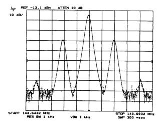
Change the modulation level, allow one sweep, and store in B with  $\bigcirc$  B.
