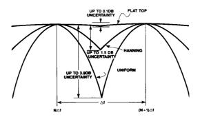
The amplitude and frequency uncertainty of the FFT display depends on the choice of the window, and the analyzer sweeptime. Amplitude uncertainty is maximum when the spectral component falls midway between the filter shapes. Passbands that are flatter in shape, like the FLATTOP filter, contribute less amplitude uncertainty, but frequency resolution and sensitivity are compromised (see TWNDOW).
