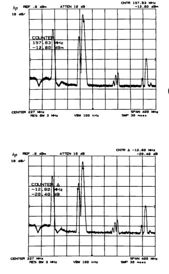
To count the difference between the signal and its neighbor, place the marker on one signal with  $\bigcirc$ ; then activate marker differential and count the next signal.
