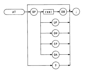
The AT command specifies the RF input attenuation from  $\emptyset$  to 70 dB, in 10 dB steps.
