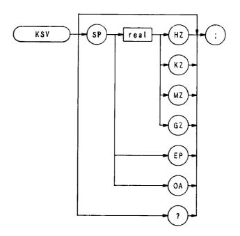
The KSV command selects a value that offsets the frequency scale for all absolute frequency readouts, such as center frequency. Relative values, like span and delta marker, are not offset.
