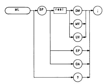
The ML command specifies the maximum signal level that is applied to the input mixer for a signal that is equal to or below the reference level.
