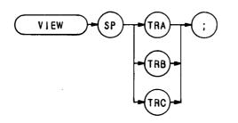
The VIEW command displays trace A, B, or C, and stops the sweep. Thus, the trace is not updated. Trace A and C are discussed below. For detailed information about trace B, see B3 in this section.
