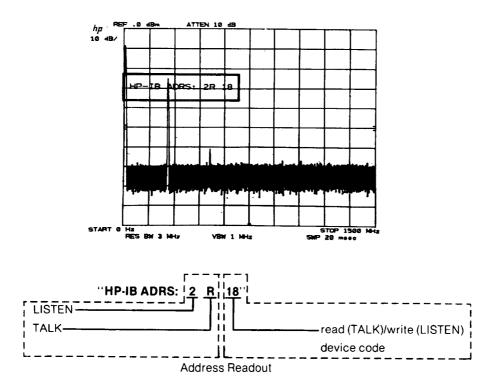
Two formats are available for addressing an HP-IB instrument or device. One command format uses separate addresses for TALKING ("R") and LISTEN ("2"). The other uses only a device code ("18") to designate the recipient of the command.
