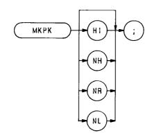
The MKPK command positions on the active marker on signal peaks.
