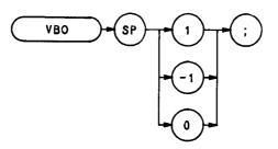
The VBO command specifies the relation between the video and resolution bandwidths that is maintained when these bandwidths are coupled. The bandwidths are usually coupled, unless the RB or VB commands have been executed.
