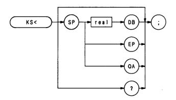
Use the KS< command when using a preamplifier at the 100 Hz to 1.5 GHz input. The KS< command offsets the amplitude readouts so the displayed amplitudes represent power levels at the preamplifier input.
