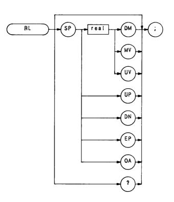
The RL command specifies the amplitude value of the top CRT graticule line, which is called the reference level. The reference level can be specified from -89.9 dBm to +30 dBm with 0.1 dB resolution.
