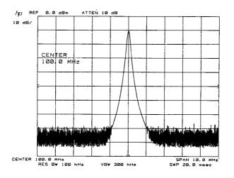
10 ASSIGN @Sa TO 718 20 PRINTER IS 701 30 DIM A(1001) 40 ! 50 OUTPUT @SA;"IP;" 60 OUTPUT @Sa;"CF100MZ;SP2MZ;S2;TS;" 70 OUTPUT @Sa;"01;TA;" 80 FOR N = 1 TO 1001 90 ENTER @Sa;A(N) 100 NEXT N 110 ! 120 FOR N = 490 TO 510130 PRINT A(N) 140 NEXT N 150 END
