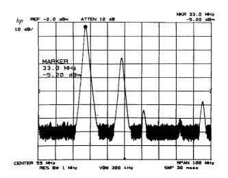
To measure the differences between this signal and any other on the display, press and use to move the second marker. The amplitude and frequency differences are read out continuously.
