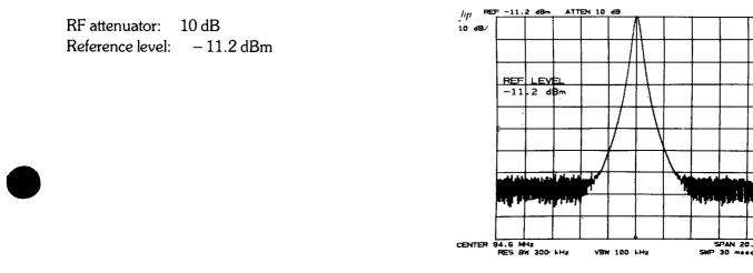
Reference level dBm units are selected with [HESET] : dBmV, dBµV, and volts referred to the analyzer's input impedance can be selected with KEY [3007] FUNCTIONS. The absolute power of the reference level remains constant when units are changed.
