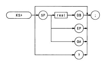
Use the KS> command when using a preamplifier at the 100 kHz to 1.5 GHz input. The KS> command offsets the amplitude readouts so the displayed amplitudes represent power levels at the preamplifier input.
