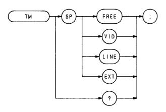
The TM command selects trigger mode: free, video, line, or external trigger. See T1, T2, T3, and T4.
