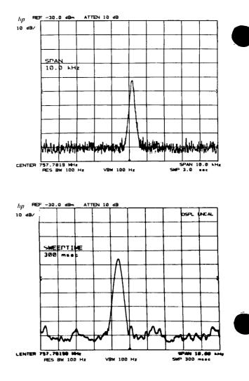
To quickly see signals present in the span, press  $( \underbrace{ state}_{max} )$  and  $( \underbrace{ } )$  several times. When the sweep completes its span, couple sweep time again with  $( \underbrace{ auto} )$ .
