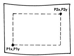
Special care must be taken to enter scaling point values which fall within the allowed scaling point range of the particular plotter being used. The following table shows the plotting ranges of each plotter exemplified here. Also shown are typical values of scaling points which can be used to give a typical plot size.
