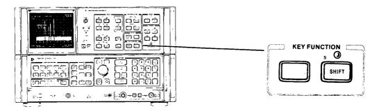
Shift functions supplement a front panel function or provide unique measurement capabilities. The  $\square \square \square$  functions are not named on the front panel but are coded by the blue characters beside the keys. For example, the frequency offset function is designated by the code V. On the front panel, the code V is found in the FUNCTION section:
