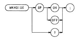
The MKNOISE command displays the RMS noise level at the marker. The RMS value is normalized to a 1 Hz bandwidth.
