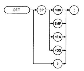
The DET command selects the kind of spectrum analyzer input detection: normal, sample, positive peak, or negative peak.
