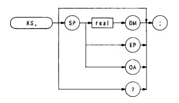
The KS, command specifies the maximum signal level that is applied to the input mixer for a signal that is equal to or below the reference level.
