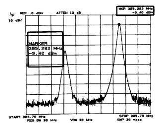
To read the left-hand signal's parameters move the marker to the signal peak with  $\bigcirc$  .
