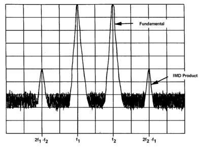
Figure 2. Two-Tone Third Order Intermodulation (Fundamentals and IMD Products)
