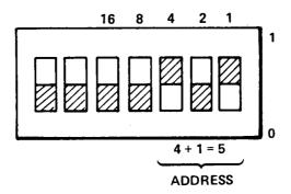
If the address switch on the plotter cannot be located, refer to the plotter's operation manual.
