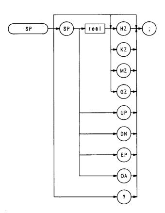
The SP command changes the total display frequency range symmetrically about the center frequency. The frequency span readout displays the total display frequency range. Divide the readout by ten to determine the frequency span per division.
