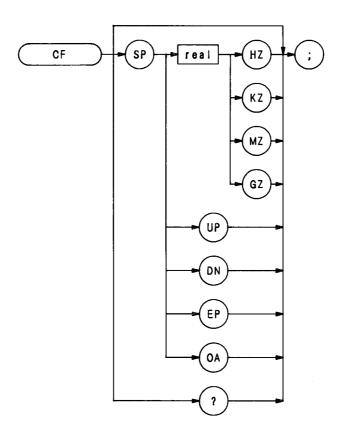
The CF command specifies the value of the center frequency, performing the same function as the front panel key. (Refer to Chapter 3 in Section I.)
