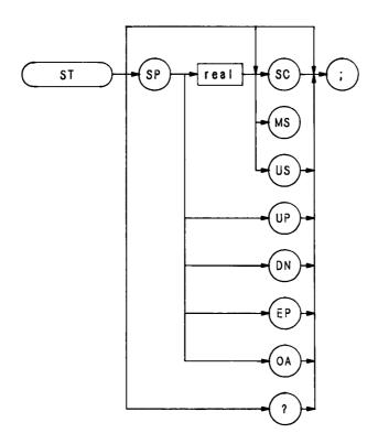
The ST command specifies the rate at which the analyzer sweeps the displayed frequency or time span.
