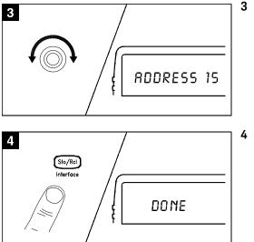
**3** Rotate the knob to view the choices on this level of the menu. When you reach the end of the list, rotate the knob in the opposite direction to view all of the other choices.
