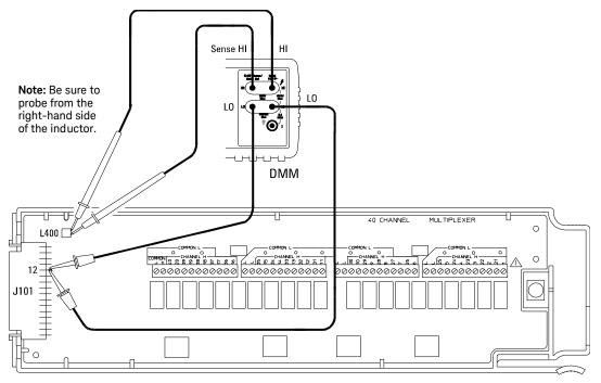
Connections for 34908A Verification Test 1
