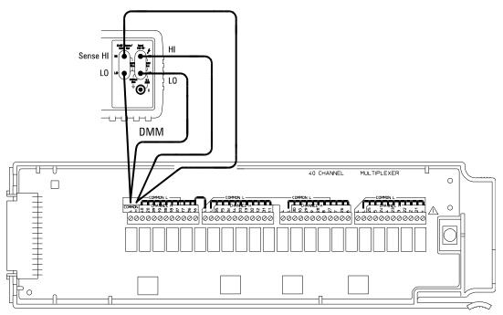
Connections for 34908A Verification Tests 4 through 43
