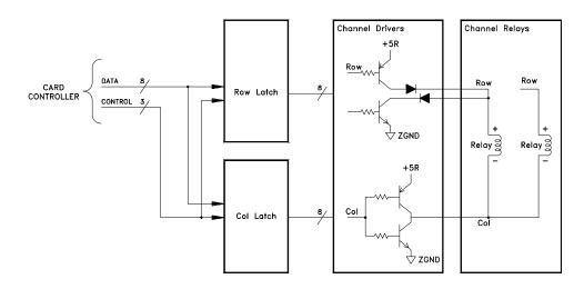
The row latch, U102, and column latch U103, control the relays. The row drivers are divided into four groups of set and reset drivers. Each group of row drivers controls eight relays. The column drivers operate as a pair. There are eight column drivers each controlling four relays. The relays are arranged in 4 rows by 8 columns.
