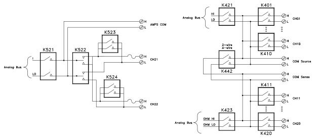
The current measurement channels are selected by relay K522. Relays K523 and K524 short the inputs when a channel is not selected. Relay K521 makes the connection to the analog bus for measurement by the Internal DMM.
