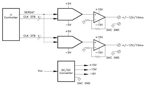
Communication with each DAC (U503 and U504) is via three lines: SERSTB, DACCLK, and SERDAT. Each DAC has a voltage output of  $\pm 3$  V. U505 and U506 amplify this voltage to the  $\pm 12$ V output.
