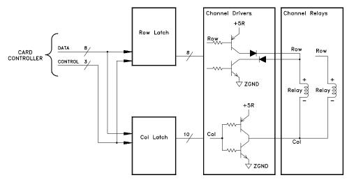
The row latch, U102, and column latches, U103 and U104, control the relays. The row drivers are divided into four groups of set and reset drivers. Each group of row drivers controls five relays. The column drivers operate as a pair. There are ten column drivers each controlling two relays.
