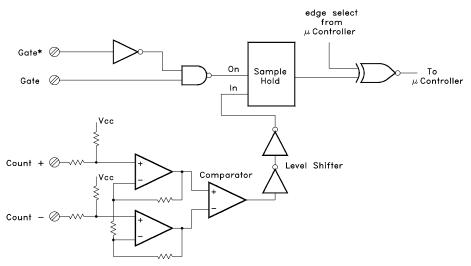
The totalizer counts signals connected to the COUNT+ and COUNT– inputs. Two op-amps, U108A and U108B, are used for input signal conditioning. Comparator U109 determines the signal trigger levels based upon the setting of the jumper at P102. With the P102 jumper in the TTL position, the totalizer counts pulses with TTL trigger levels. With the jumper at P102 in the AC position the trigger level is at zero.
