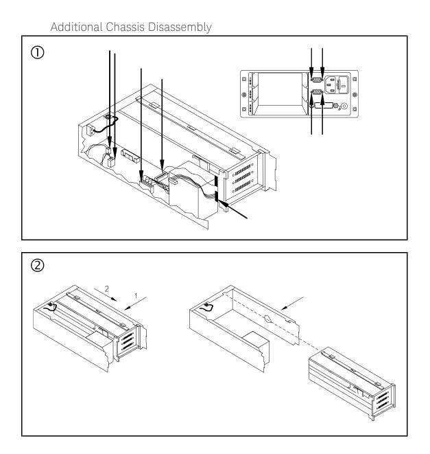
Plug-In Module Disassembly
