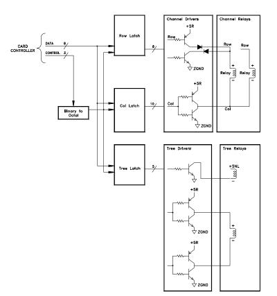
The row latch, U102, and column latches, U103 and U104, control the relays. The row drivers are divided into four groups of set and reset drivers. Each group of row drivers controls five relays. The column drivers operate as a pair. There are ten column drivers each controlling two relays. The analog bus backplane relays are non-latching.
