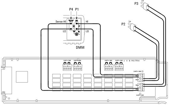
Connections for 34904A Verification Tests
