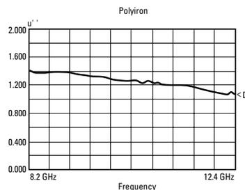
Examine the properties of materials across the RF and microwave frequency spectrum.
