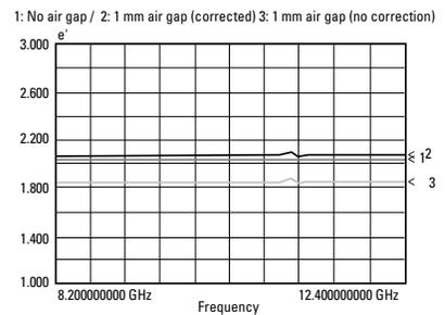
**Traditional methods produce spurious data at periodic frequencies. With the HP 85071B you get accurate data at all frequencies.**
