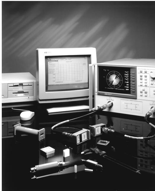
Small samples of the material under test (MUT) are machined to fill the cross section of coaxial or waveguide transmission lines and measured within the fixture. Or large, flat samples are placed between antennas and measured under free space conditions.
