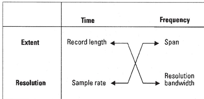
**Figure 2. Some measurements have both time-domain and frequency-domain aspects. Because of the nature of the fast Fourier transform, these two aspects are not independent. The extent and resolution of the time and frequency data are interrelated as shown here.**
