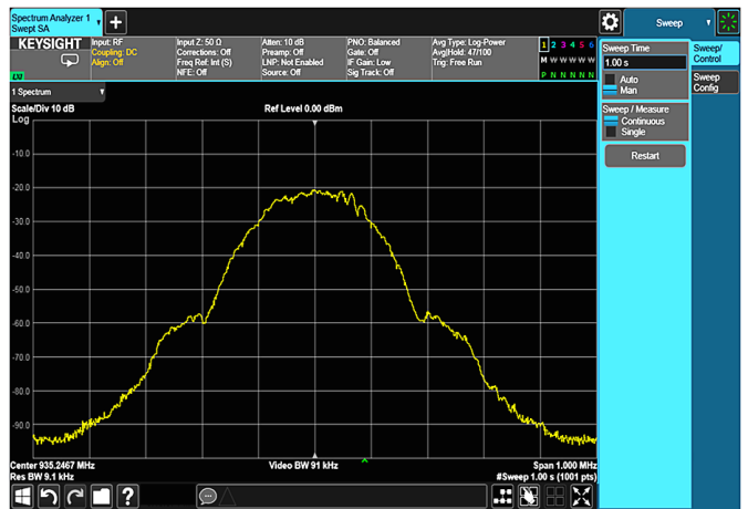
Figure 2-39. Spectrum of time slot 3 reveals that the spurious signal is not caused by this burst.
