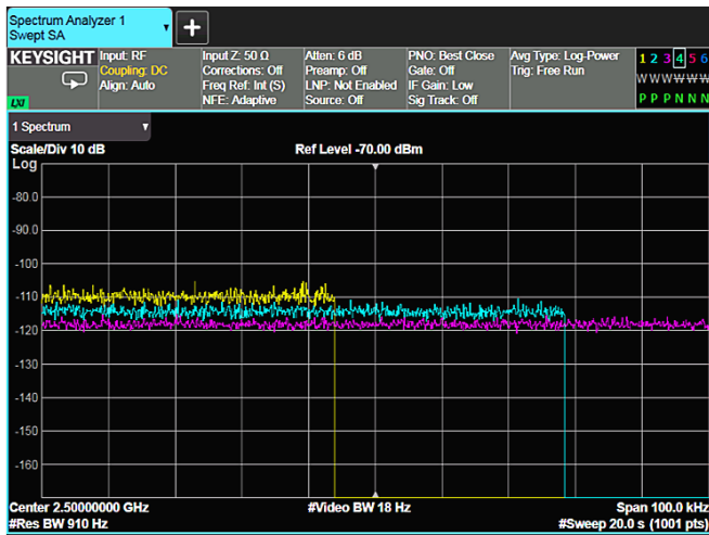
Figure 2-30a. Positive peak detection mode: reducing video bandwidth lowers peak noise but not average noise.
