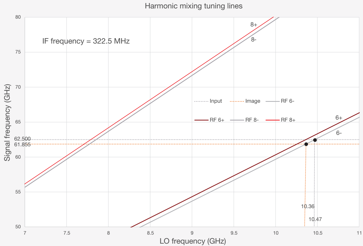
Figure 7-16 Harmonic tuning lines for the X-Series analyzers using the M1970 Series mixers
