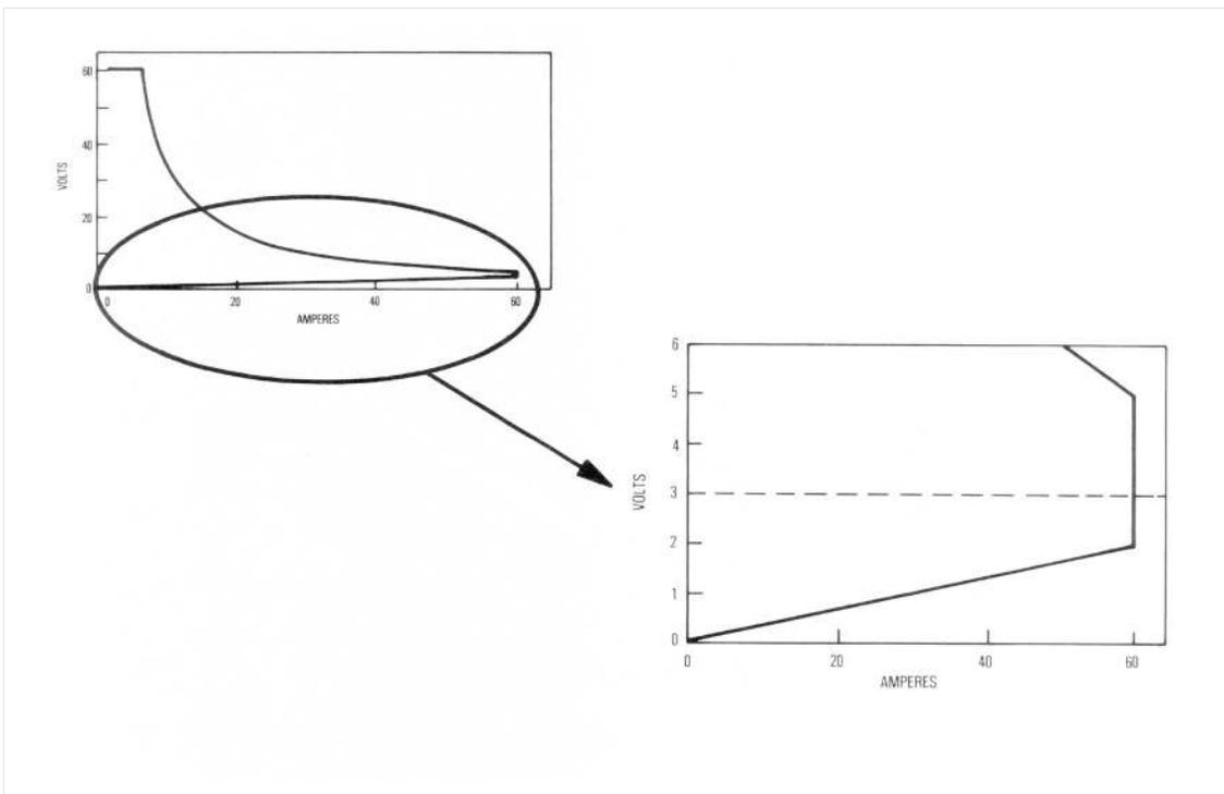
Figure 8. Operating Characteristics of a Keysight Electronic Load
