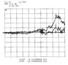
Figure 13 Measurement of typical repeatability using a ground-signal probe. Three S<sub>11</sub> measurements of an on-wafer short circuit (referenced to an initial measurement stored in the memory of the HP 8510) are shown: (#1) System noise floor, contact unbroken between stored and current measurement, (#2) on-wafer contact broken by raising probe and then recontacting, (#3) on-wafer contact broken by raising probe shifting laterally 1 mil and then recontacting.
