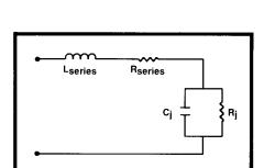
Figure 7 Simple diode model
