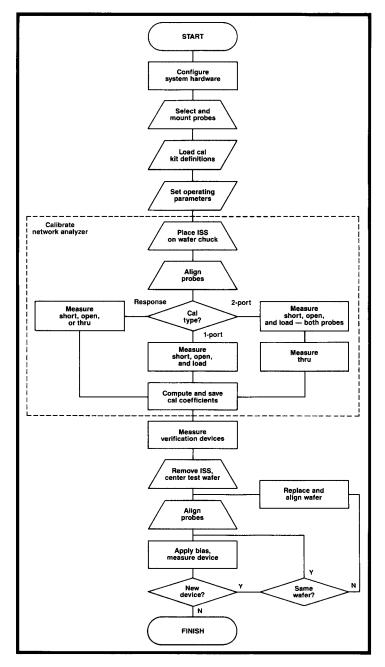
Figure 4 Flow diagram for a typical measurement of an on-wafer device using the Cascade Microtech Model 42 manual probe Station and the HP 8510 network analyzer system.
