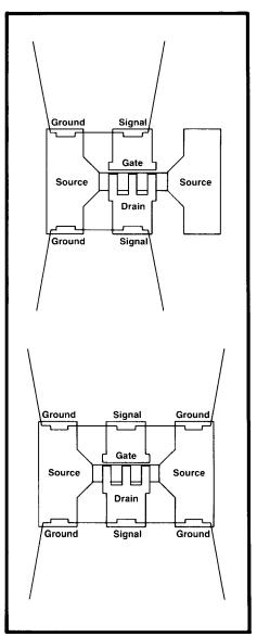
Figure 12 Recommended probe and pad configuration for making probed on-wafer measurements with a network analyzer:
