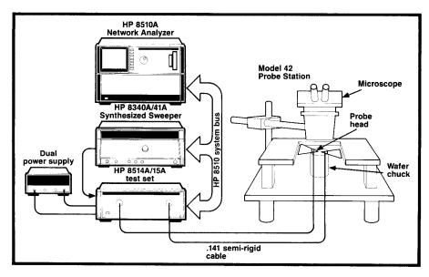
Figure 1 System Block Diagram and Equipment List
