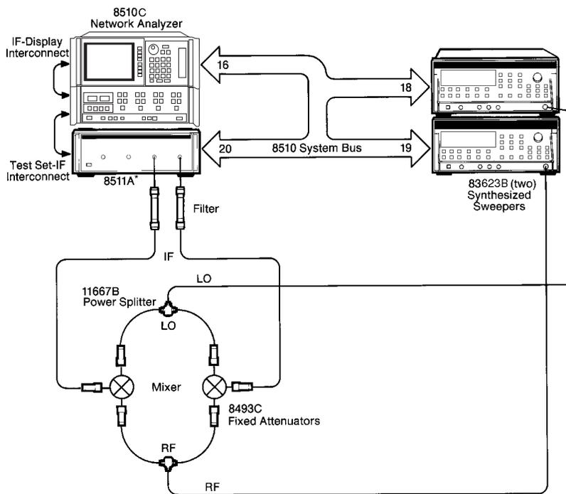
Figure 1. 8510C mixer test system
