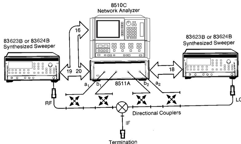
Figure 7. Mixer input impedance and isolation measurement system.
