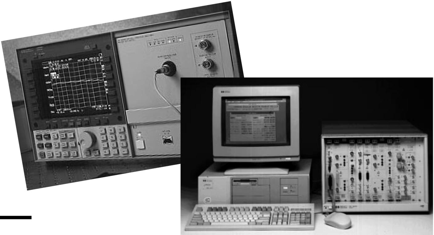
Used as a tunable, bandwidth-variable filter for the HP 75000 Series 90 modular telecom analyzer, the HP 71451B optical spectrum analyzer's monochromator allows access to individual channels of a WDM signal for BERT measurements.
