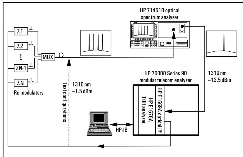
The monochromator output on the HP 71451B optical spectrum analyzer allows the user access to the channel of interest, giving full control over the wavelength and resolution bandwidth while preserving the input signal's state of polarization.
