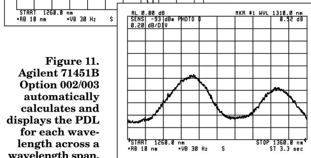
**Figure 11.** Agilent 71451B Option 002/003 automatically calculates and displays the PDL for each wavelength across a wavelength span.
