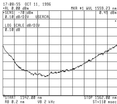
**Figure 15. PDL of a material probe**
