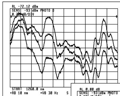
**Figure 10.** Agilent 71451B Option 002/003 automatically traces maximum and minimum power points measured during a swept PDL measurement.
