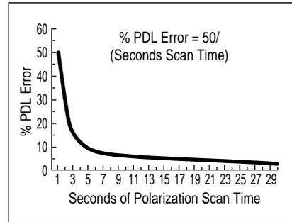
**Figure 7. Typical Agilent 8153A/11896A PDL polarization scan time uncertainty contribution (for power measurement averaging time T=20 msec only)**
