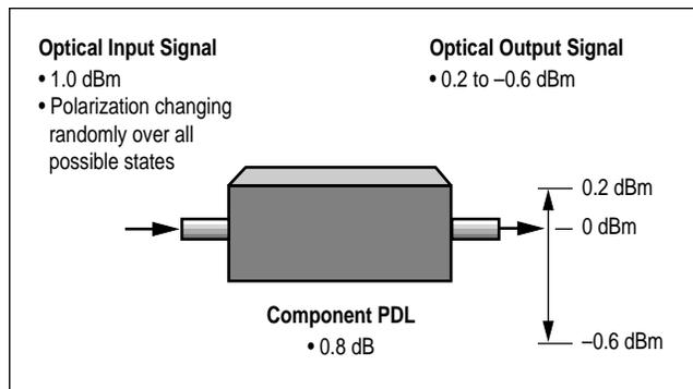
**Figure 1. Polarization-dependent loss causes power variations.**
