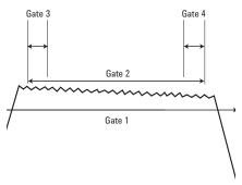
Figure 15. On this GSM pulse, powerful data configuration routines during four gate times, provide the feeds for the display.
