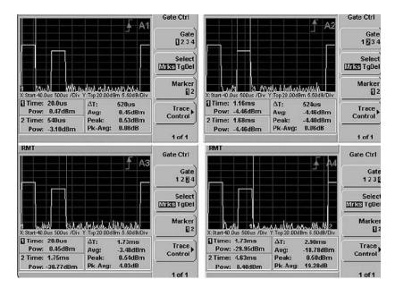
Figure 9. Measurement flexibility with four independent time gates
