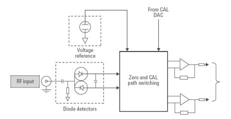
Figure 6. Internal zero and cal block diagram
