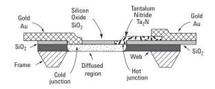
Figure 3. Cross section of Keysight thermocouple chip, where power dissipated in the tantalum-nitride resistor heats the hot junction.
