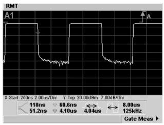
Figure 8. Large color display with automatic power and time measurements
