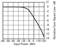
Figure 4. The diode detection characteristic is square law from the noise level up to -20 dBm, followed by a transition region and then a linear range to +20 dBm. The lower graph shows deviation from "square-law."
