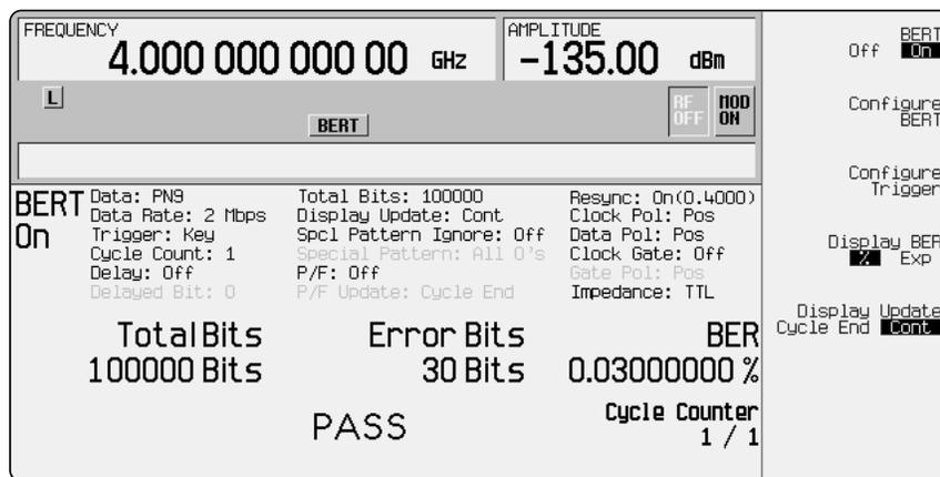
Figure 16. BER analyzer display
