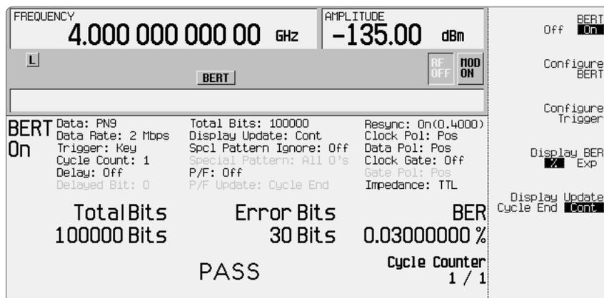
Figure 6. Agilent ESG-D series RF signal generator BERT user interface
