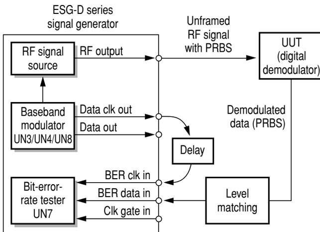
Figure 12. Unframed signal test configuration
