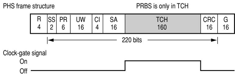
**Figure 9. PHS frame structure and clock-gate signal**
