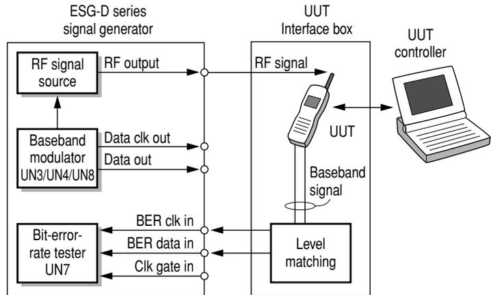
Figure 10. Typical test configuration
