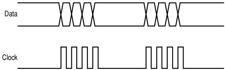
**Figure 7. Bursted data and clock**
