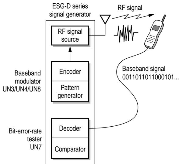
**Figure 5. Agilent ESG-D BERT configuration**
