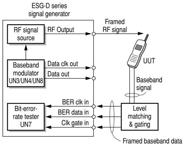
Figure 11. Gated test configuration
