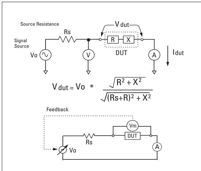
Figure 6. Applied Signal and Constant Level Mechanism
