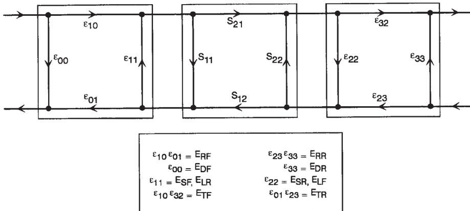
Figure 15. 8-term TRL\* error model and generalized coefficients
