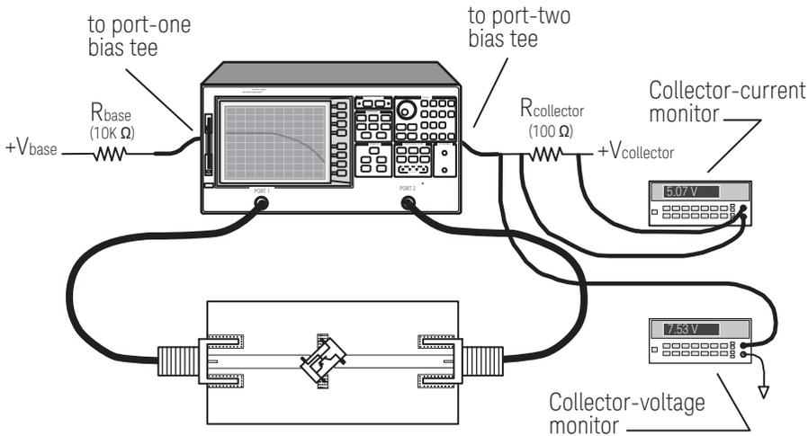
Figure 24. Two-port calibration was performed prior to taking S-parameter data of the transistor.
