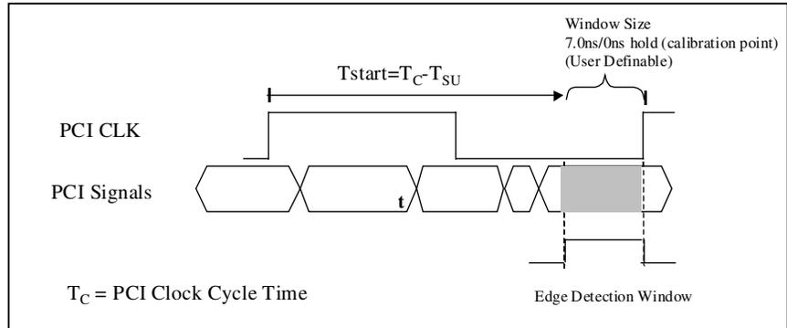
Figure 3: Calculation of Measurement Window Start
