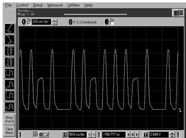
**Step 6:** View the pulse signal on a 54845A Infiniium Oscilloscope.
