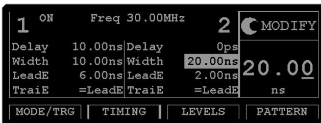
**Step 3:** Set the frequency, width and delay values for the WRITE, ERASE pulses in the TIMING menu.
