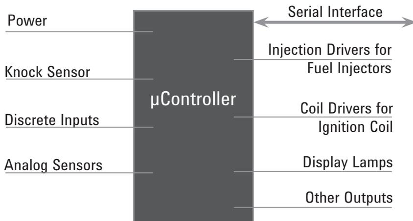
Figure 7. Serial interface for engine control ECM
