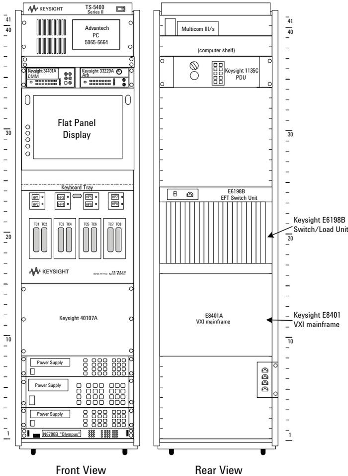
Figure 3. VXI/GPIB Express Connect (front and rear views)
