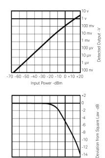
Figure 1. The diode detection characteristic ranges from the square-law region through a transition region to linear detection.
