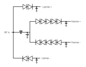
Figure 2. Schematic of the diode-attenuator-diode sensing element
