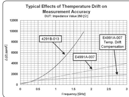
Figure 20. Effect of the temperature drift compensation function
