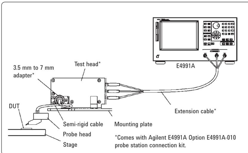
Figure 17. Probe measurement configuration using E4991A Option E4991A-010
