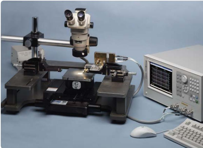
Figure 16. Agilent E4991A with probe station
