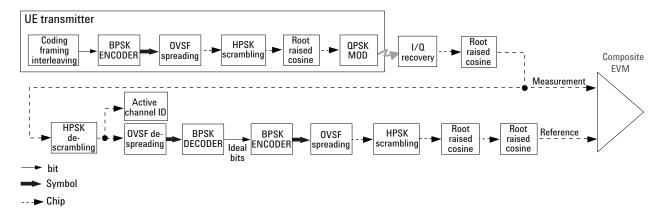
Figure 23. Process to calculate the composite EVM
