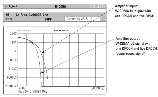
Figure 18. CCDFs for a W-CDMA signal with a DPCCH and five DPDCH, with and without compression
