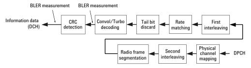
Figure 35. BER and BLER measurements in the DL for a DPCH.
