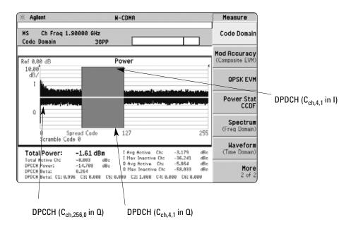
Figure 28. Code domain power measurement for the UL 768 kbps reference measurement model (one DPCCH and two DPDCHs). Signal with high LO instability
