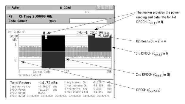
Figure 27. Code domain power of W-CDMA UL signal with a DPCCH and three DPDCHs
