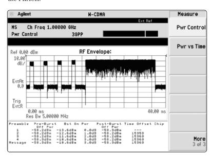
Figure 14. Open loop power control measurement
