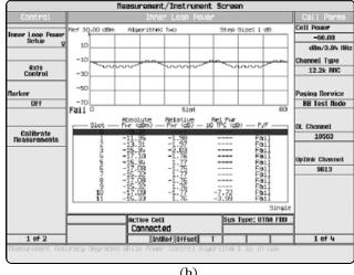
Figure 15. Inner loop power control measurement example (a) using a spectrum analyzer (a signal generator was used to provide the power control commands) and (b) using a one-box tester
