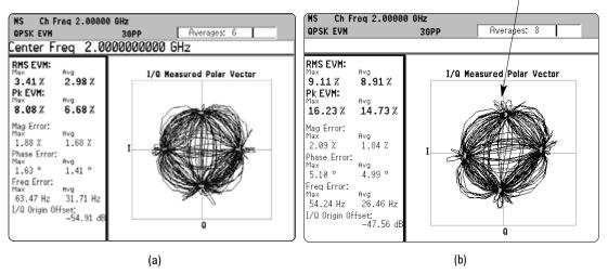
Figure 22. Vector diagram and QPSK EVM measurement for an UL W-CDMA signal (one DPDCH and one DPCCH at the same amplitude level). (a) Transmitter without any impairment. (b) Transmitter with an I/Q quadrature error
