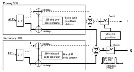
Figure 38. Physical structure for P-SCH and S-SCH
