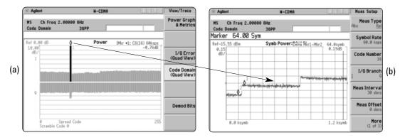
Figure 32. (a) Code domain power measurement of a W-CDMA UL signal with the DPCCH and one DPDCH at 60 kbps ( $C_{ch,64,16}$ ) and (b) symbol EVM measurement for the DPDCH ( $C_{ch,64,16}$ )
