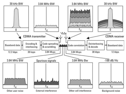
Figure 1. CDMA transmission and reception processes
