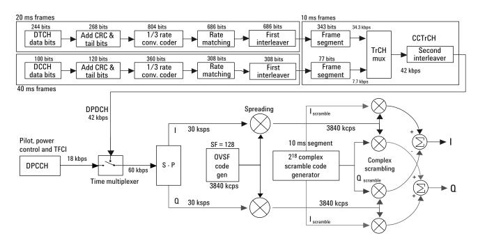
Figure 10. Downlink DPDCH/DPCCH coding, spreading, and scrambling. (For an alternative description, refer to [2], [9], and [10])
