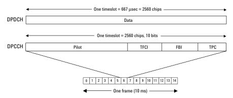
Figure 9. Uplink slot structure of a DPDCH and a DPCCH
