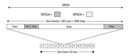
Figure 7. DPCH (DPDCH/DPCCH) slot and frame structure
