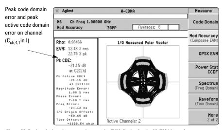
Figure 29. Peak code domain error and composite EVM display for the UL 768 kbps reference measurement model (one DPCCH and two DPDCHs). Signal with high LO instability
