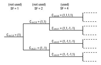
Figure 25. Code tree generation of OVSF codes [3]
