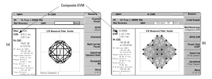
Figure 24. Composite EVM and vector diagram for a signal with (a) UL 12.2 kbps reference measurement channel (one DPDCH and a DPCCH), and (b) three DPDCHs and a DPCCH
