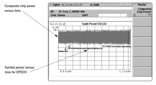
Figure 33. Chip power versus time for a W-CDMA UL signal with the DPCCH and one DPDCH at 60 kbps  $(C_{ch.64.16})$ , combined with symbol power versus time for the DPDCH  $(C_{ch.64.16})$
