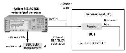
Figure 37. Test setup for BER/BLER using recovered baseband bits
