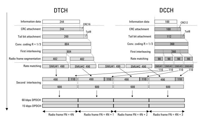
Figure 40. Channel coding of UL reference measurement channel (12.2 kbps)
