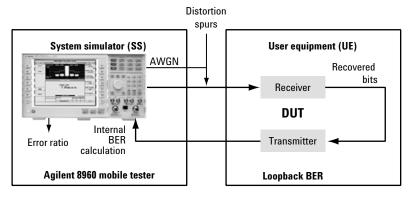
Figure 36. Basic test setup for BER loopback test
