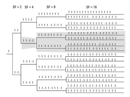
Figure 26. Effects of using variable SFs
