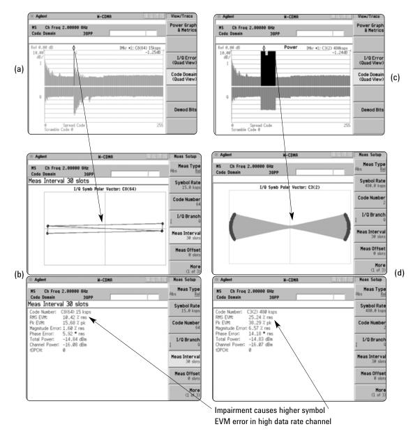
Figure 31. (a) Code domain power measurement of a W-CDMA UL signal with the DPCCH and one DPDCH at 15 kbps ( $C_{\mathrm{ch},256,64}$ ) and (b) symbol EVM measurement for the DPDCH at 15 kbps ( $C_{\mathrm{ch},256,64}$ ). (c) Code domain power measurement of a W-CDMA UL signal with the DPCCH and one DPDCH at 480 kbps ( $C_{\mathrm{ch},8,2}$ ) and (d) symbol EVM measurement for the DPDCH at 480 kbps ( $C_{\mathrm{ch},8,2}$ )
