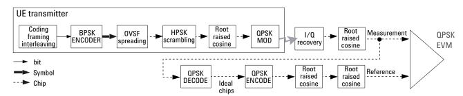
Figure 21. Process to calculate QPSK EVM for a W-CDMA UL signal
