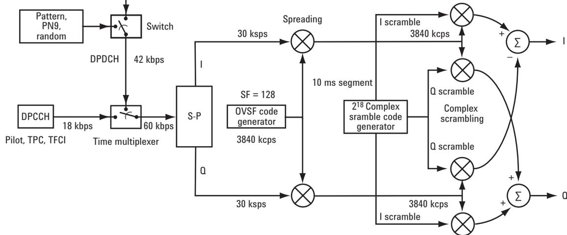
**Uplink 3GPP W-CDMA block diagram outlining the difference between the arbitrary waveform playback and real-time W-CDMA modes. The real-time capability encompasses the entire block diagram. The arbitrary waveform playback provides only the lower, unshaded portion of the block diagram. Both are included in Option 400.**
