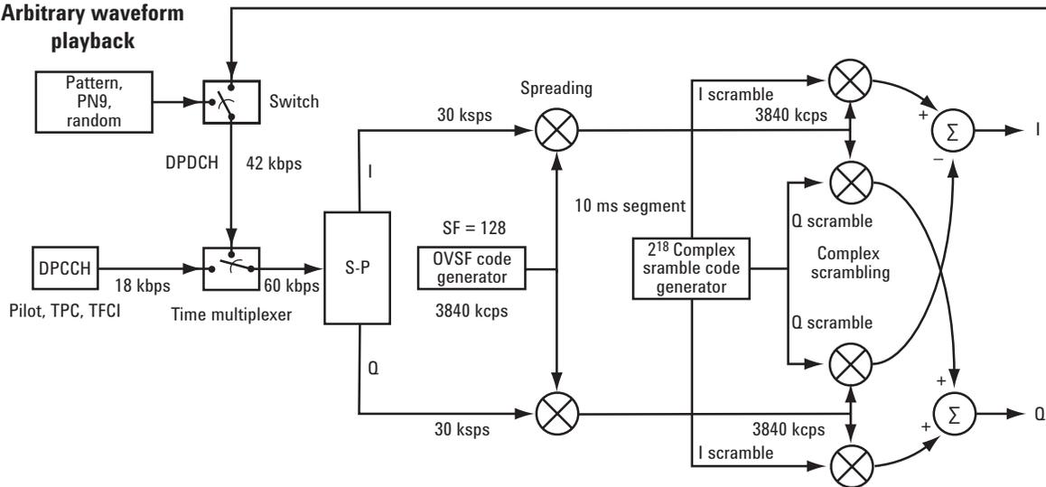
**Downlink 3GPP W-CDMA block diagram outlining the difference between the arbitrary waveform playback and real-time W-CDMA modes. The real-time capability encompasses the entire block diagram. The arbitrary waveform playback capability provides only the lower, unshaded portion of the block diagram. Both capabilities are included with Option 400.**
