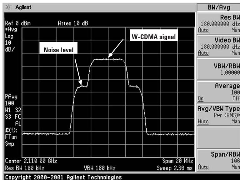
Add calibrated AWGN to the W-CDMA signal by setting  $C/N$ ,  $E_b/N_c$ , or  $E_c/N$
