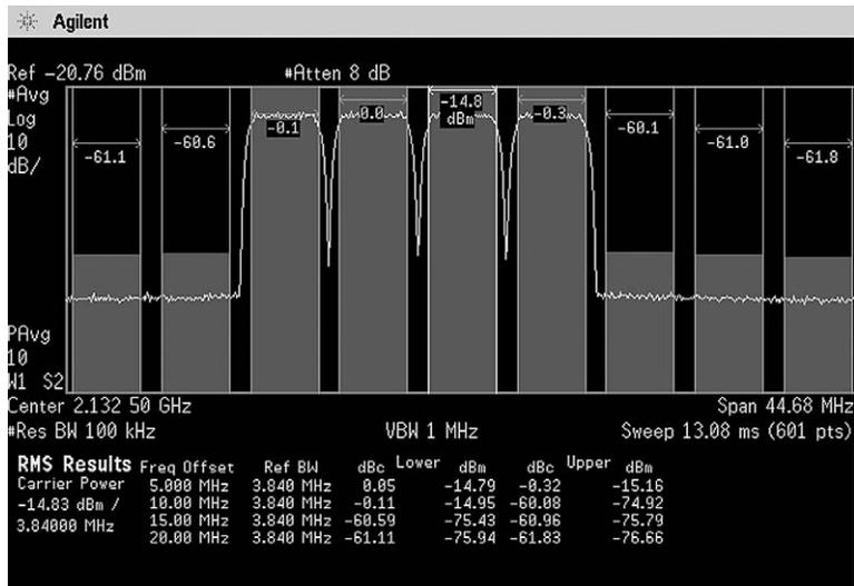
The signal is composed of four 3GPP W-CDMA carriers using Test Model 1 with 64 DPCH.
