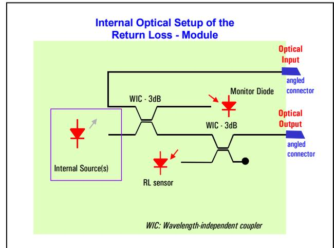
Figure 6: Optical Setup in the Return Loss Module.
