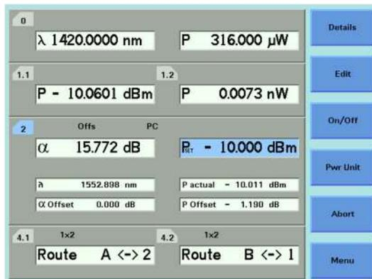
Figure 2. Instrument display showing power control parameter and calibrated effective wavelength of attenuator module.
