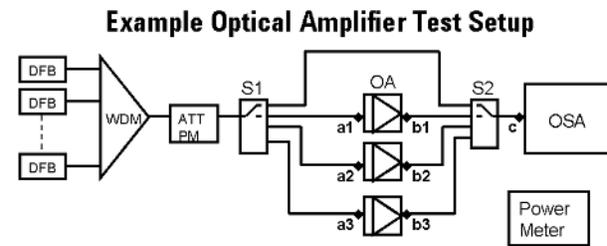
Figure 1. Basic setup for optical amplifier test with adjustable multichannel input power. In this case, 3 amplifiers are connected at the same time. (The abbreviations are: DFB, distributed feedback laser, e.g. Keysight 81662A; WDM, wavelength-dependent multiplexer; ATT PM, attenuator with power control, e.g. 81577A; S1 and S2, switches, e.g. 81595A; OA, optical amplifier; OSA, optical spectrum analyzer, e.g. 86146B; optical power meter, e.g. 81630B.)
