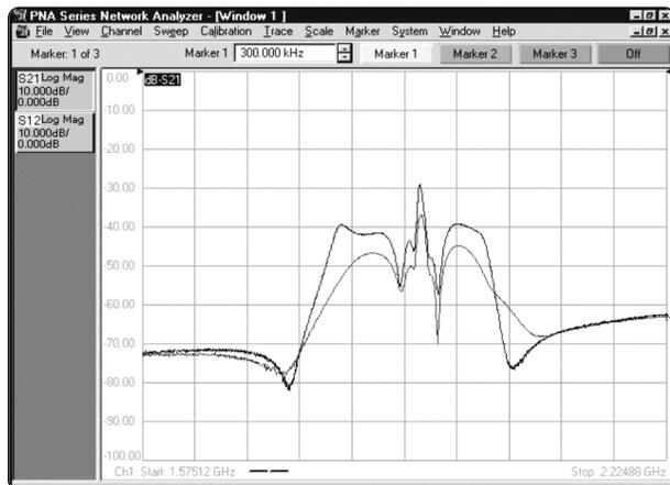
Figure 5: Isolation measurement with open and loaded duplexer third port
