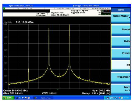
Figure 5c. Two tone signal created on a vector signal generator showing nearly 70 dBc from the two tones to the third-order products.
