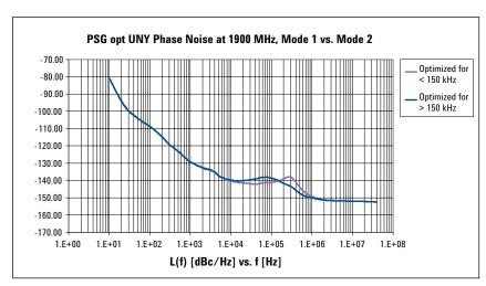
Figure 8a. Adjust the phase lock loop bandwidth to optimize the phase noise.
