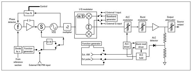
Typical vector signal generator block diagram.
