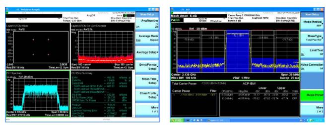
Figure 7c. 5 MHz E-TM 1.1 signal with baseband filter and symbol rolloff length = 20 Ts.
