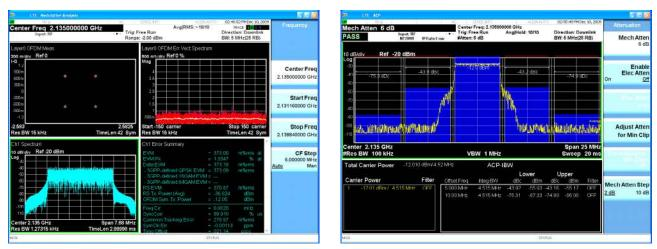
Figure 7b. 5 MHz E-TM 1.1 signal without baseband filter and symbol rolloff length = 20 Ts (best EVM).
