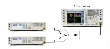
Figure 5b. Three-resistor combiner used to isolate the outputs of the sources.
