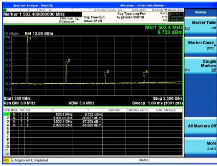
Figure 1a. Harmonic distortion measurement using a signal analyzer.
