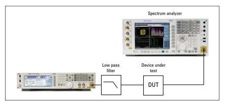
Figure 1b. The harmonic distortion of a signal source improved by installing a low pass filter at the source's output.
