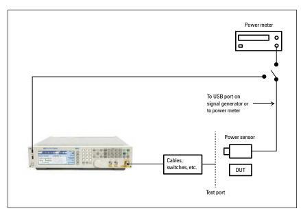
Figure 2. Setup for improving level accuracy of the signal.
