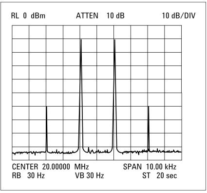
Figure 5a. Example of intermodulation products caused by two sources intermodulating with each other.
