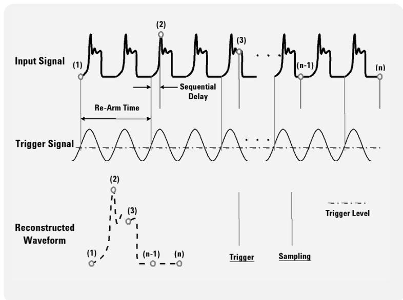
Figure 2. An equivalent time oscilloscope acquires each datum after a different trigger pulse.
