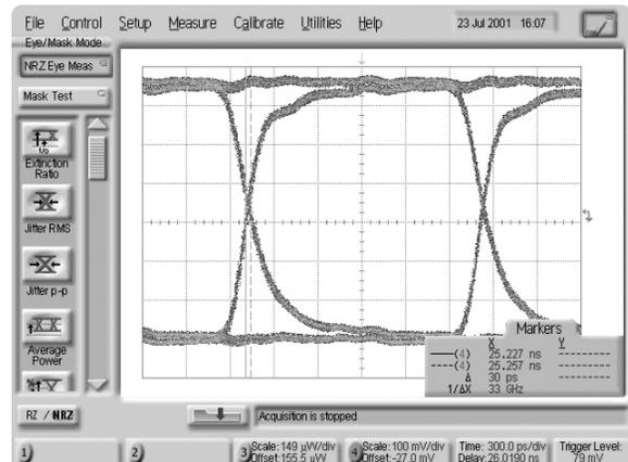
Figure 6. A wide loop bandwidth results in a very clean measurement of the signal.
