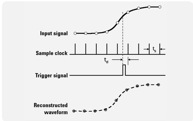
Figure 1. A real-time scope acquires several data points after each trigger pulse.
