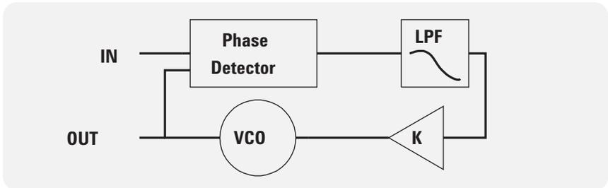
Figure 3. A simple PLL schematic.
