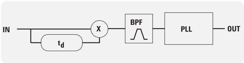
Figure 4. A simple CDR circuit using a hard delay, a band-pass filter, and a PLL.
