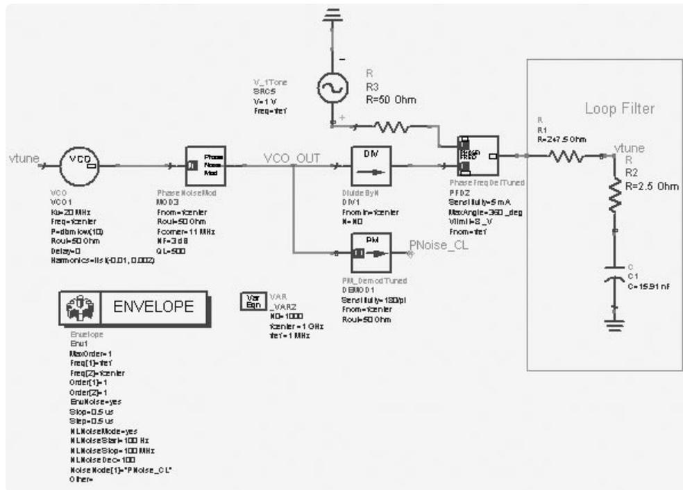
Figure B. 1 - A simple PLL model in Agilent ADS with a passive lead-lag loop filter.
