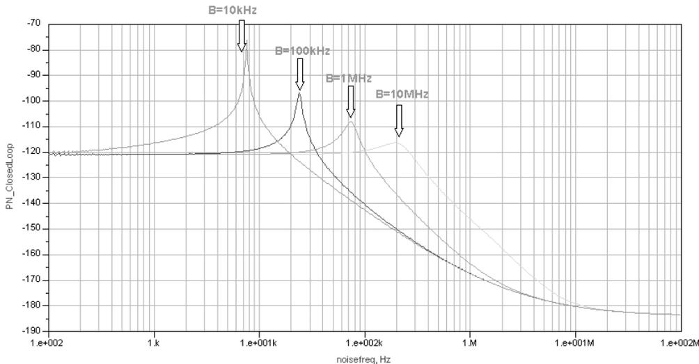
Figure B. 2 - The output phase noise of the PLL in Figure A.1 is related to the loop bandwidth of the filter. The different shapes of the curves are due to the change in damping factor with the change in filter parameters.
