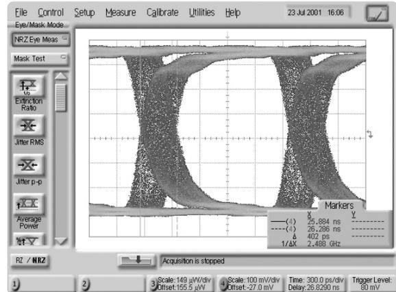
Figure 5. A narrow loop bandwidth results in a more accurate representation of the jitter.
