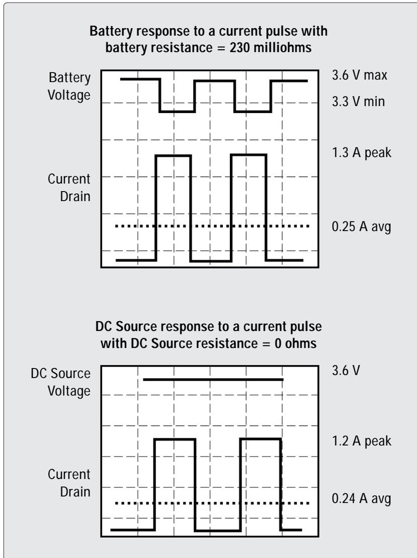
**Figure 4.** A GSM mobile phone performs differently when powered by a power supply with zero output resistance than when powered by an actual battery, making battery operating time appear longer than it would under realistic conditions.
