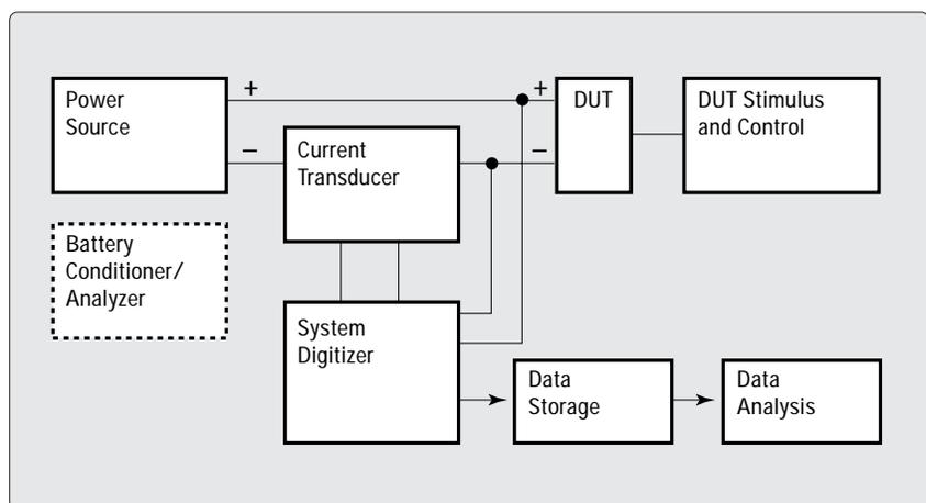
Figure 2. A generic system for battery current-drain measurement and analysis
