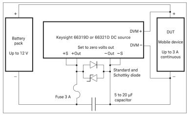
Figure 1. Recommended test set-up
