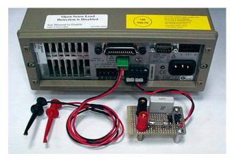
Figure 2. Example of an external protection network and DVM leads  $\,$
