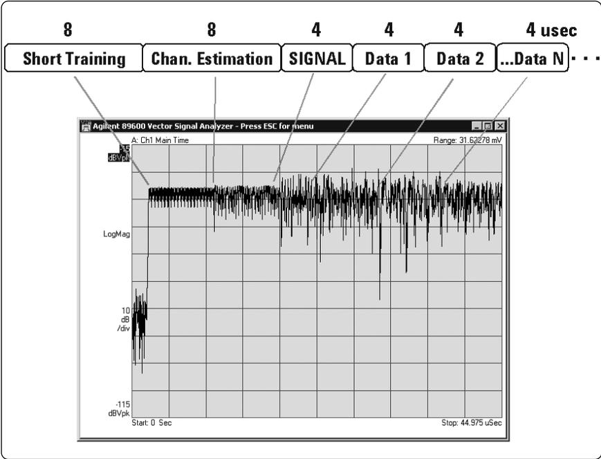
Figure 1. Structure of an OFDM burst or frame
