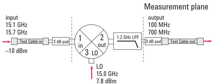
Figure 1. Example of a mixer-under-test configuration.
