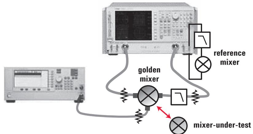
Figure 10. 8720ES group delay configuration using golden and reference mixers.
