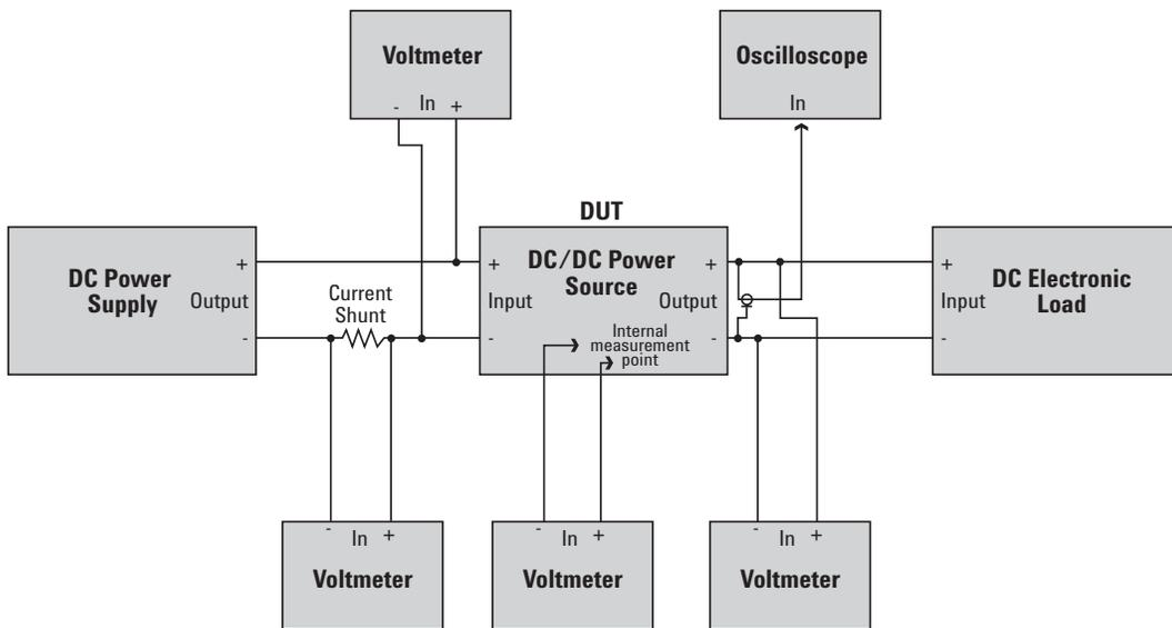
The test system diagrammed in **Figure 4** is just one example of a manual setup for testing some aspects of the design. Other R&D engineers would have other manual setups on their benches to test for other parameters. In this case, the total R&D manual test system is actually distributed throughout the benches of the entire design team.
