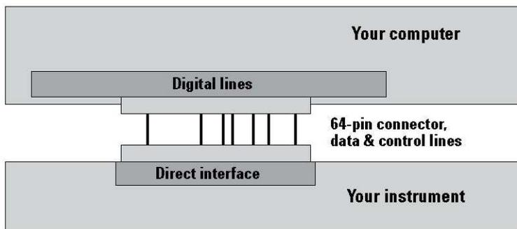
Figure 1. Early instrument control utilized hard-wired commands.
