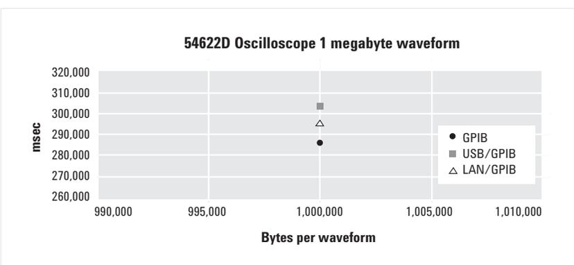
Figure 5. Data transfer time for 1 megabyte waveform
