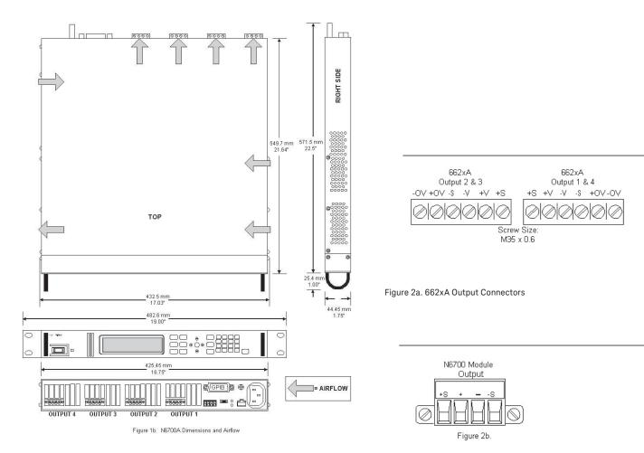
Figure 1b. N6700A/B Dimensions and Airflow
