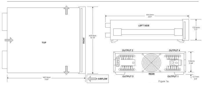
Figure 1a. 662xA Dimensions and Airflow
