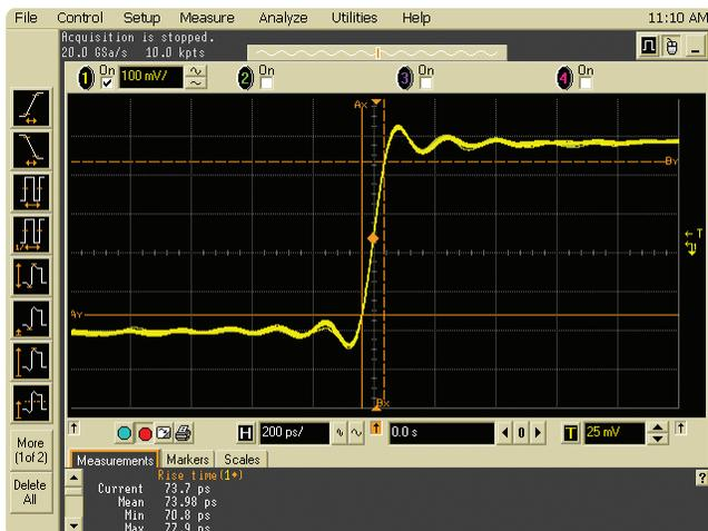
Figure 11. Risetime measurement without bandwidth-enhancement
