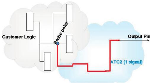
*The thick lines show the routes added by ATC2 timing cores.*
