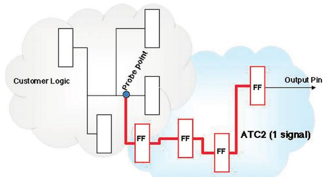
*The thick lines show the FF's and routes added by ATC2. Since there is a FF "in the fabric" in addition to one at the I/O, timing impact on your design is minimized.*
