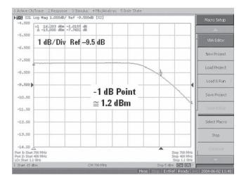
Figure 14. Example of conversion compression measurement
