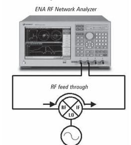
Figure 15. Examples of isolation measurement configurations
