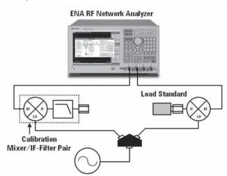
Figure 3. Setup for the vector mixer characterization
