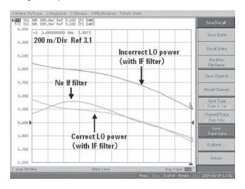
Figure 12. SWR measurement example
