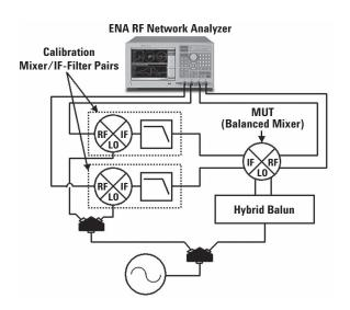
Figure 23. Balanced mixer measurement configuration
