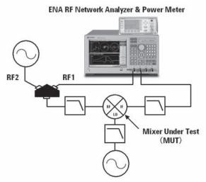
Figure 18. Example of intermodulation distortion measurement configuration
