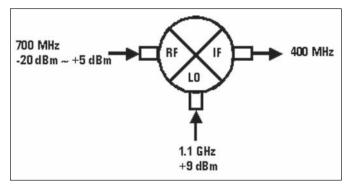
Measurement parameters of the network analyzer, the external signal source, and the power meter should be set in advance, prior to performing the conversion compression measurement. For the external signal source setting, see Appendix 3, "Setup for the External Signal Source". For the power meter setting, see Appendix 4, "Setup for the Power Meter".
