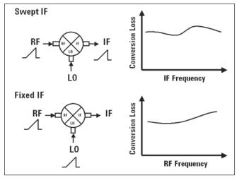
Figure 8. Conversion loss measurements
