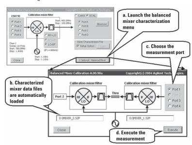
Figure 24. Balanced mixer characterization menu
