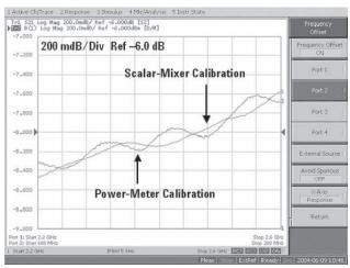
Figure 11. Conversion loss measurement comparison (SMC vs. Power Cal.)
