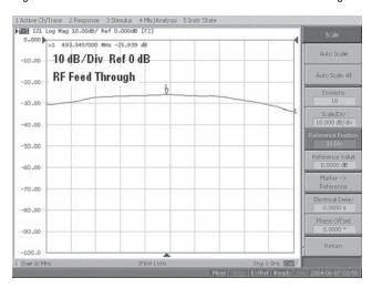
Figure 17. Example of RF feed through measurement
