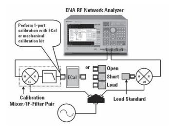
Figure 4. Calibration mixer/IF-filter pair characterization
