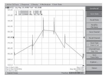
Figure 19. Example of two-tone third-order intermodulation distortion measurement)
