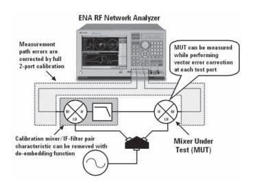
Figure 2. Overview of vector-mixer calibration
