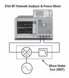
Figure 6. Configuration of the scalar-mixer calibration
