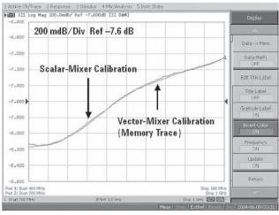
Figure 9. Comparison of conversion loss measurement results (VMC vs. SMC)
