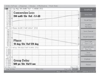
Figure 10. Conversion loss measurement example with VMC
