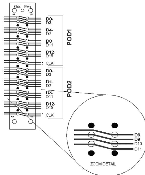
**Figure 7.** Here, a soft touch connectorless probe observes the bus signals. The reduced probe loading and the ability to route directly through the landing pattern makes for an acceptable logic analyzer connection.
