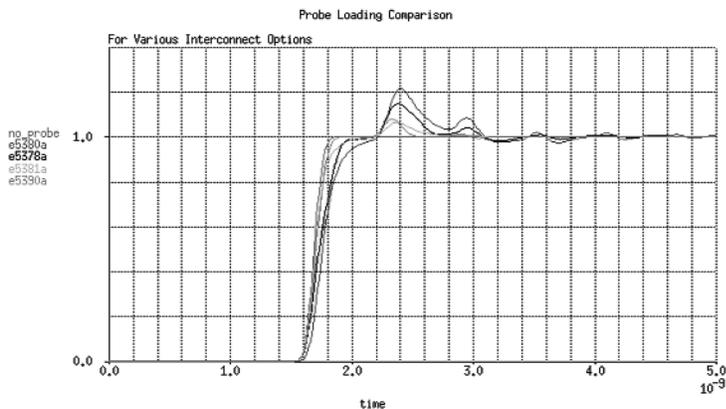
Figure 2. Waveforms are a good way to compare probe loading for various interconnect options. As the connector size is reduced (or removed), the loading decreases. The original rise time in this system is 150 ps.
