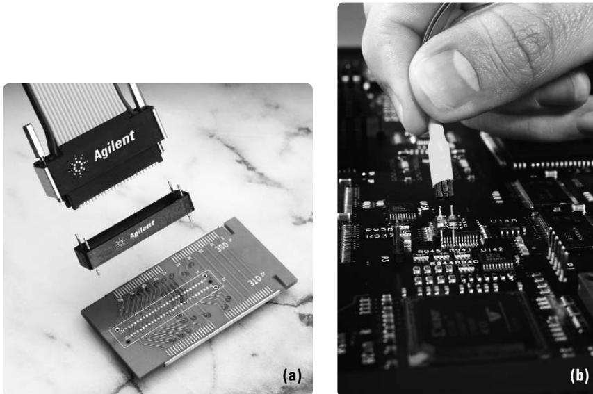
**Figure 1.** These photos compare a “designed-in” versus an “after-the-fact” probe. The Agilent E5390A shows the connection scheme for the new soft touch connectorless probe (a). In this case the user must put the landing pads in the initial design. The Agilent E5381A shows a possible connection method for a signal that didn’t have predefined testability (b).
