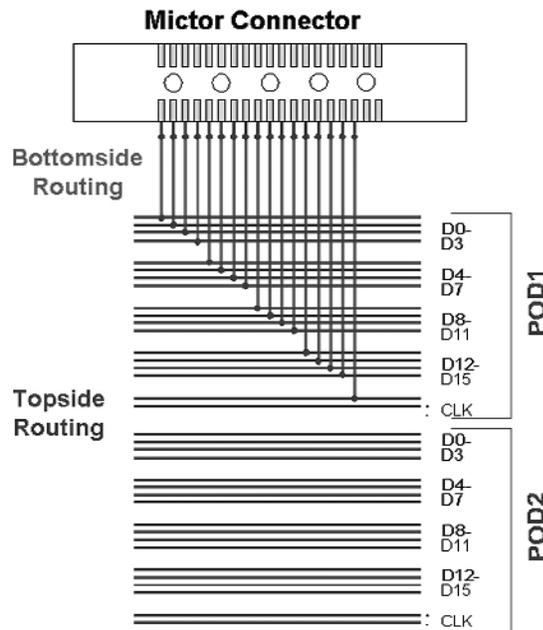
**Figure 6.** This connection scheme uses a Mictor connector-based probe to observe bus signals. Notice the additional trace length needed to connect to the Mictor. This trace capacitance is added to the connector (3 pF). The net capacitance of this connection is greater than 3.5 pF, resulting in system failure.
