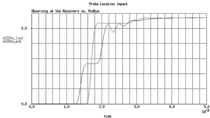
**Figure 3.** For a series-terminated system, the waveforms are observed at the receiver and the probe tip. Notice the stair-step shape of the wave when observed in the middle of the line. This shows the forward-traveling, half-amplitude wave that's moving toward the receiver. The waveform reaches its final value when the reverse traveling reflection is super-imposed upon the forward-traveling wave.
