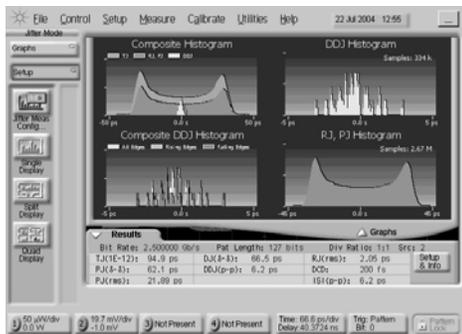
Fig. 5: Jitter decomposition of the stressed eye signal at 2.5 GHz
