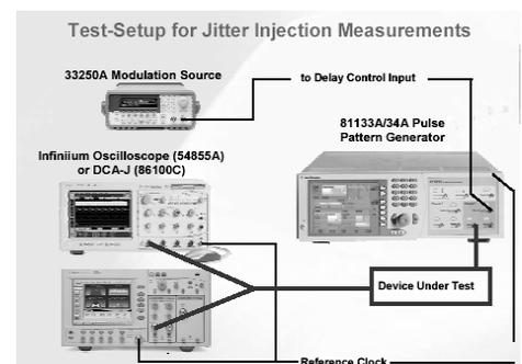
Fig. 4.: Jitter insertion setup
