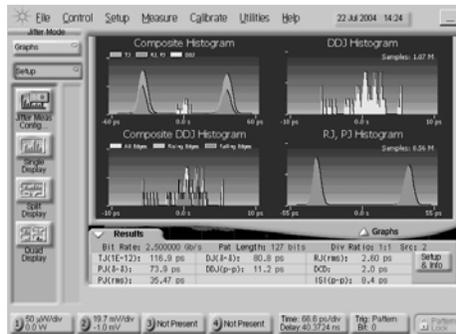
Fig. 7: Jitter decomposition of the bi-modal waveform at 2.5 GHz
