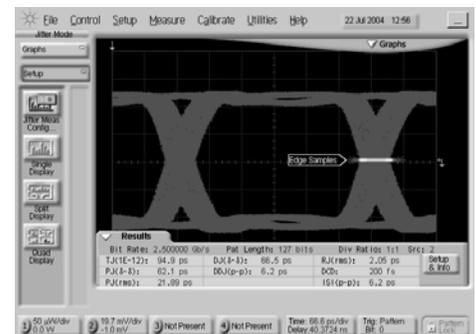
Fig. 3: Stressed eye (low-jitter stimulus plus sinusoidal jitter) at 2.5 GHz
