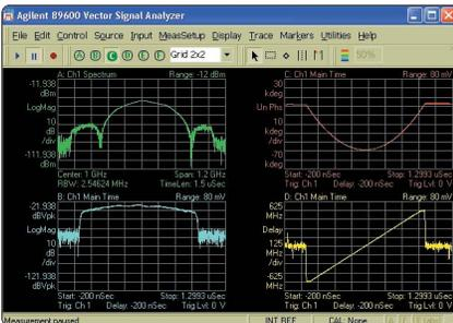
Figure 4. Chirp radar signal up to 1 GHz wide
