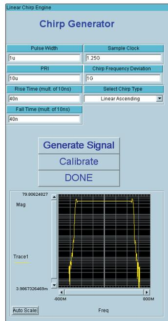
Figure 6. Linear chirp generator parameter entry screen
