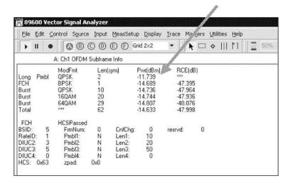
Figure 7. Downlink subframe power measurements
