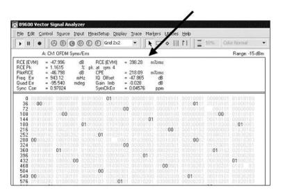
Figure 10. Numeric display of RCE results
