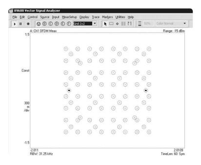
Figure 5. Keysight 89600 IQ measurement of WiMAX downlink frame
