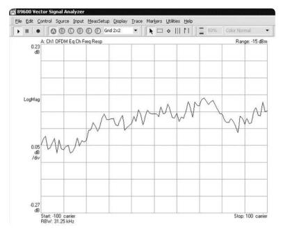
Figure 8. Spectral flatness or channel frequency response with the Keysight 89601A
