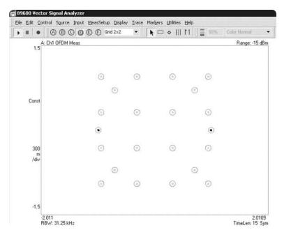
Figure 9. Graphical display of IQ constellation
