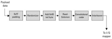
Figure 4. Channel coding
