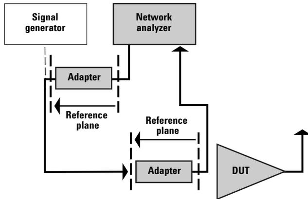
**Figure 5.** When calibrating paths such as signal-generator-to-DUT-input, adapter de-embedding moves the reference plane away from the network analyzer, ensuring characterization of just the signal path
