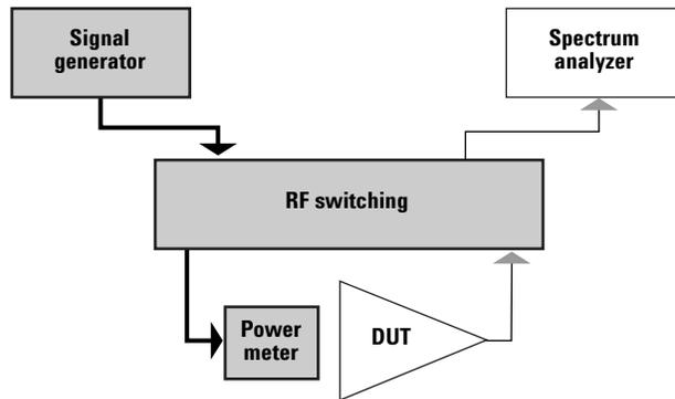
**Figure 6.** By substituting a power meter at the DUT input, you can measure loss through the input path.
