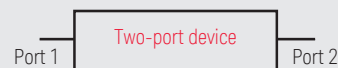
Figure 1. Modeling the RF signal path as a two-port device provides the S-parameters needed for calibration and correction
