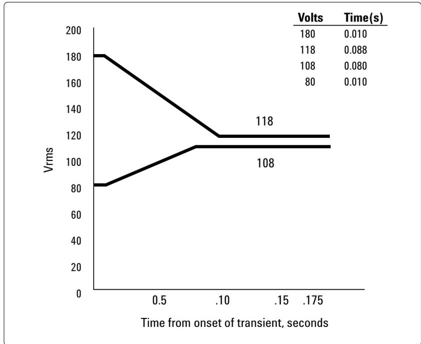
Figure 1 Envelope of normal AC voltage limits
