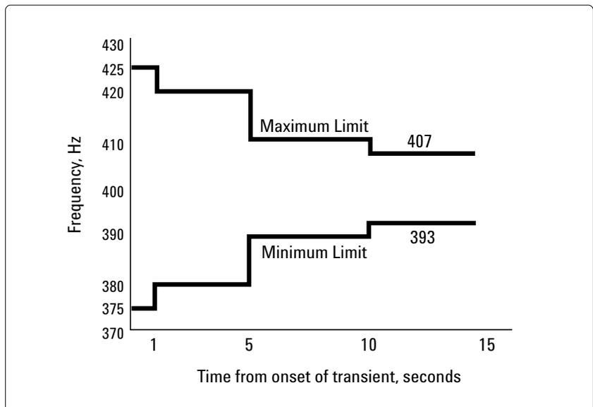
Figure 2 Envelope of normal AC frequency limits
