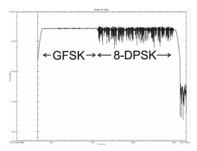
Figure 5a. Power versus time measurement for an EDR packet showing the GFSK and 8-DPSK modulated sections of the packet.) This waveform was captured using the Keysight Technologies N4017A Graphical Measurement Application (GMA) with Option 205 for *Bluetooth* EDR testing)
