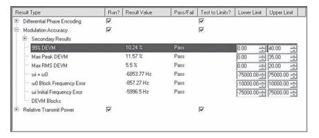
Figure 9. Measurement of the DEVM modulation accuracy for a *Bluetooth* EDR packet; also shown are the carrier frequency stability measurements over the entire packet
