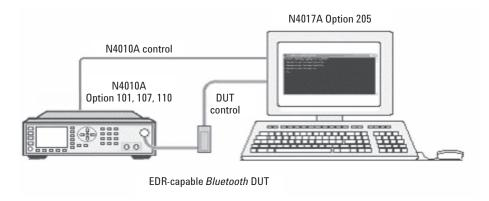
Figure 7. Measurement configuration for testing a *Bluetooth* EDR radio using the Keysight N4010A test set and N4017A Graphical Measurement Application
