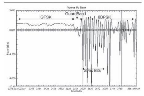
Figure 5b. Power versus time waveform displaying the transition between GFSK and 8DPSK modulation schemes
