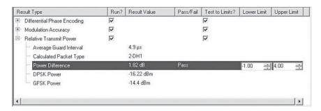
Figure 8. Measurement of the relative transmit power for an EDR packet using  $\pi/4\text{-}DQPSK$  modulation
