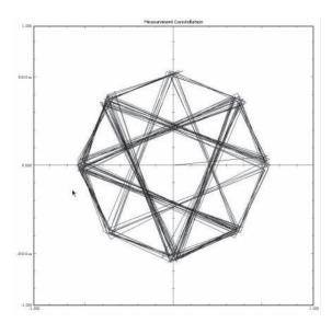
Figure 6. Measurement constellation of an EDR payload using a  $\pi/4\text{-}D\Omega\text{PSK}$  modulation
