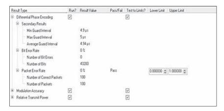
Figure 11. Measurement of the packet error rate and bit error rate for an EDR waveform
