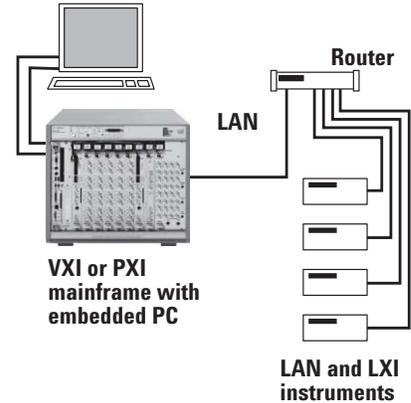
**Figure 4.** An embedded PC with a LAN port can be used as the system controller in a hybrid VXI/LXI or PXI/LXI system.
