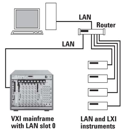
Figure 3. Add a LAN slot-0 card to a VXI mainframe to create a LAN-based hybrid VXI/LXI system.
