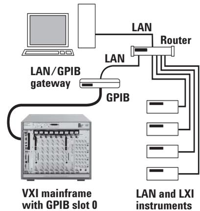
Figure 2. A router plus a LAN/GPIB gateway enables creation.
