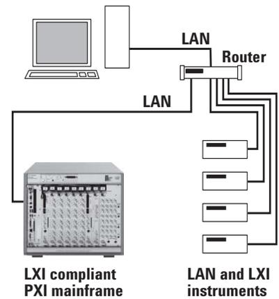
**Figure 5.** An LXI-compliant mainframe brings the benefits of PXI switching to a hybrid PXI/LXI system.
