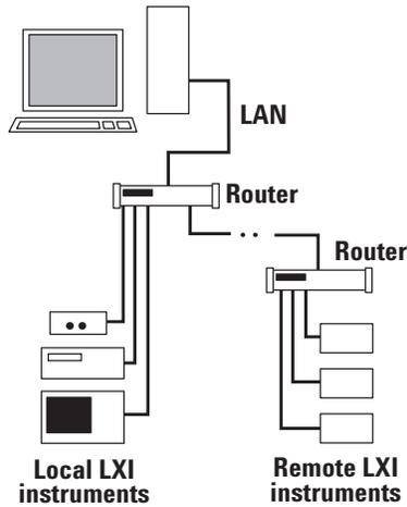
**Figure 6.** Using multiple routers enables easy connection of local and remote LXI devices to a PC's LAN port.
