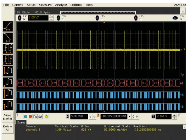
Figure 2. memory depth of up to 128 Mpts allows for the capture of high resolution analog and digital waveforms
