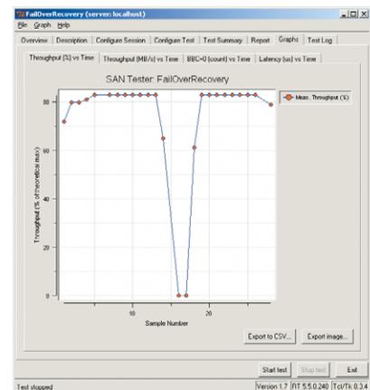
Figure 3 - Failover recovery test
