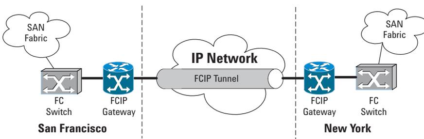
Figure 1. FCIP tunneling between two separate FC SAN islands.
