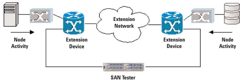
Figure 2. SAN Tester creating stress load on extension system.
